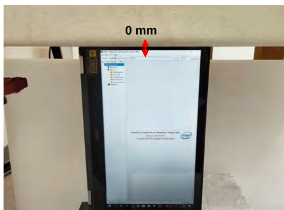
Fig.7 EUT Left side to flat phantom
