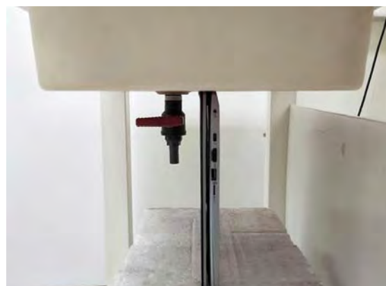
Fig.5 EUT Bottom side to flat phantom
