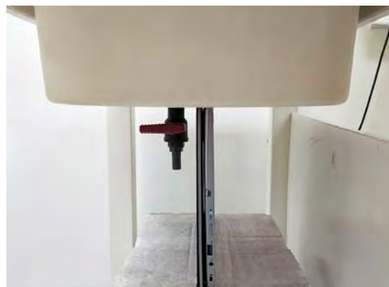
Fig.4 EUT Top side to flat phantom
