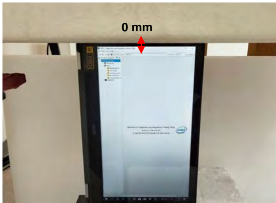
Fig.7 EUT Left side to flat phantom
