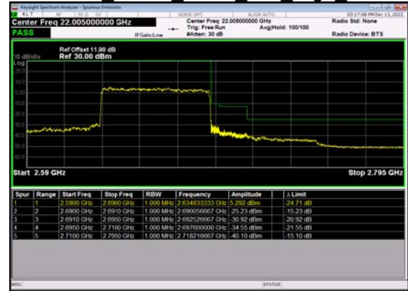
N41(60M)_DFT-s- OFDM QPSK Outer Full High CH
