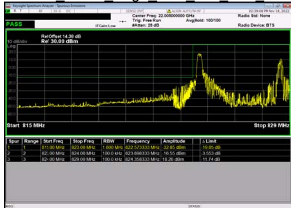
N5(10M)_DFT-s- OFDM BPSK Edge 1RB Left Low CH
