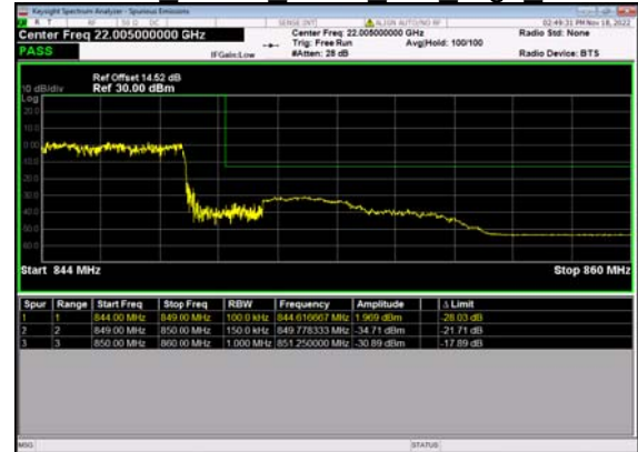
N5(15M)_DFT-s- OFDM QPSK Outer Full High CH
