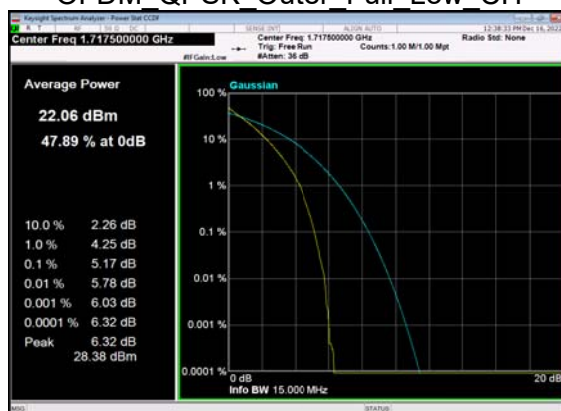
N66(15M)_DFT-s-OFDM QPSK Outer Full Low CH
