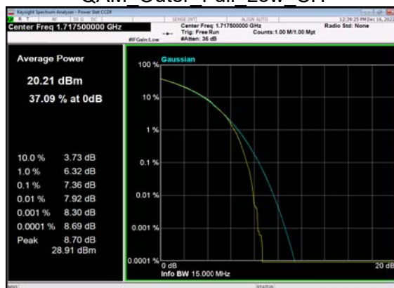
N66(15M)_CP-OFDM_16QAM Outer Full Low CH
