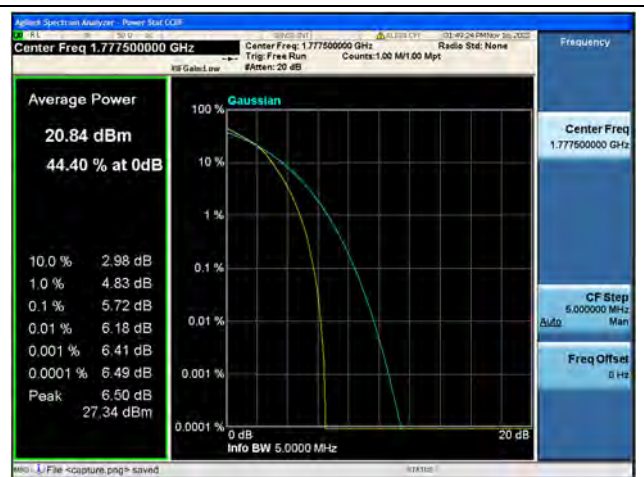
Band66 / 5MHz / High CH / 16QAM
