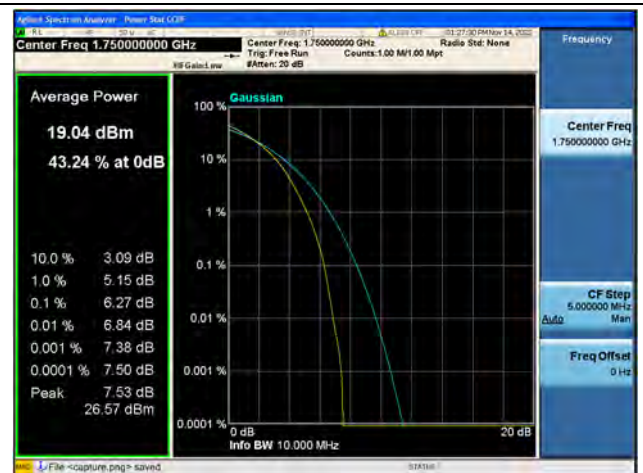
Band4 / 10MHz / High CH / 64QAM
