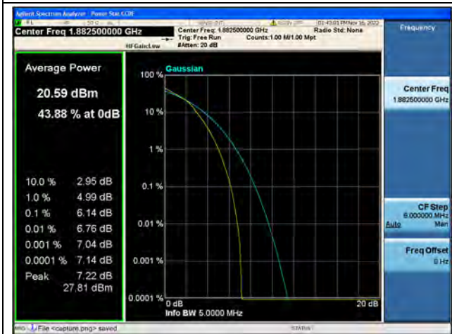
Band25 / 5MHz / Mid CH / 16QAM
