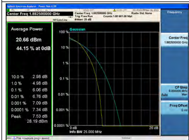
Band25 / 15MHz / Mid CH / 16QAM
