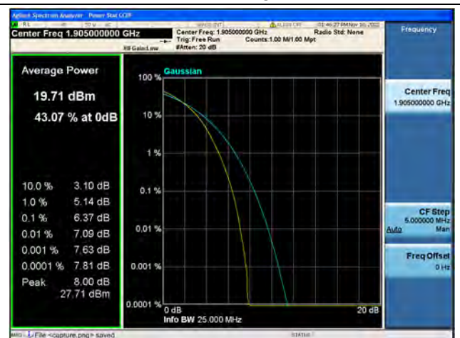
Band25 / 20MHz / High CH / 64QAM
