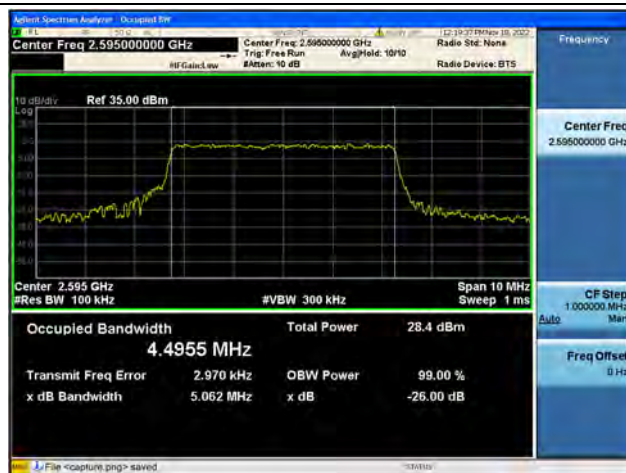
Band38 / 5MHz / 16QAM/ Mid CH
