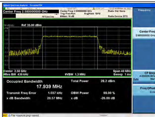
Band38 / 20MHz / 16QAM/ Low CH
