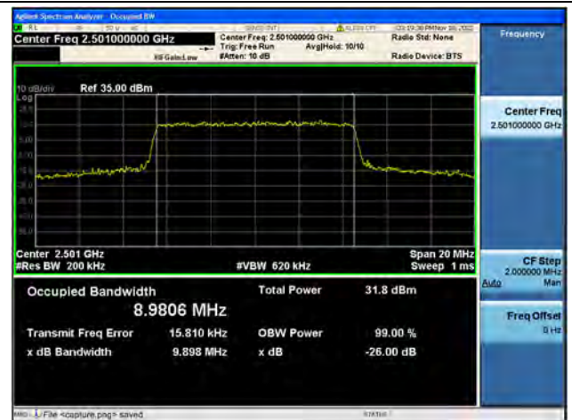
Band41 / 10MHz / QPSK/ Low CH
