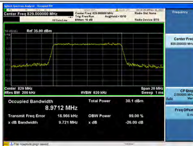
Band26Part22 / 10MHz / 16QAM/ Low CH
