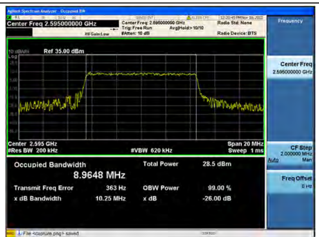
Band38 / 10MHz / 16QAM/ Mid CH
