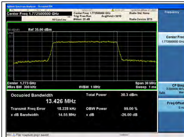
Band66 / 15MHz / QPSK/ High CH
