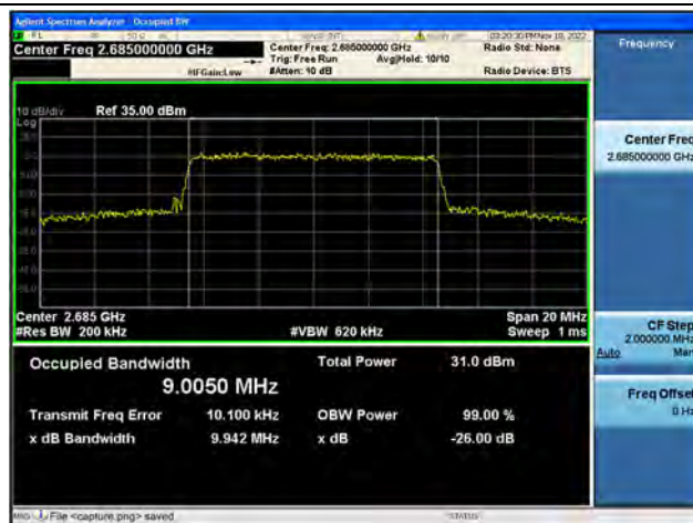
Band41 / 10MHz / 16QAM/ High CH
