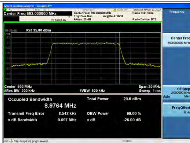
Band71 / 10MHz / 16QAM/ High CH
