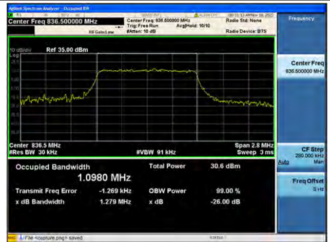
Band26Part22 / 1.4MHz / QPSK/ Mid CH
