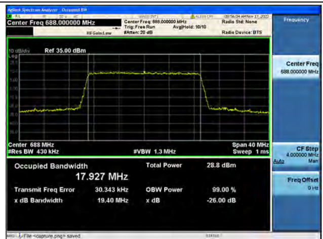
Band71 / 20MHz / 64QAM/ High CH
