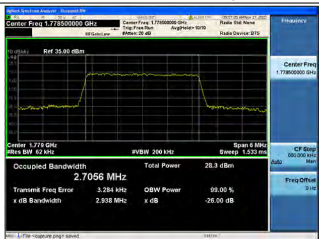
Band66 / 3MHz / 64QAM/ High CH
