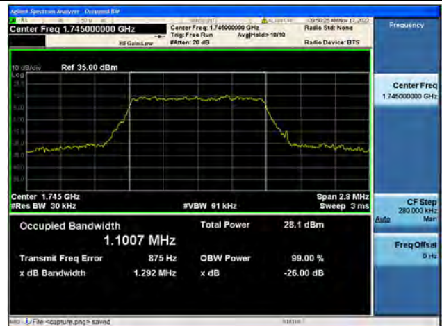
Band66 / 1.4MHz / 64QAM/ Mid CH
