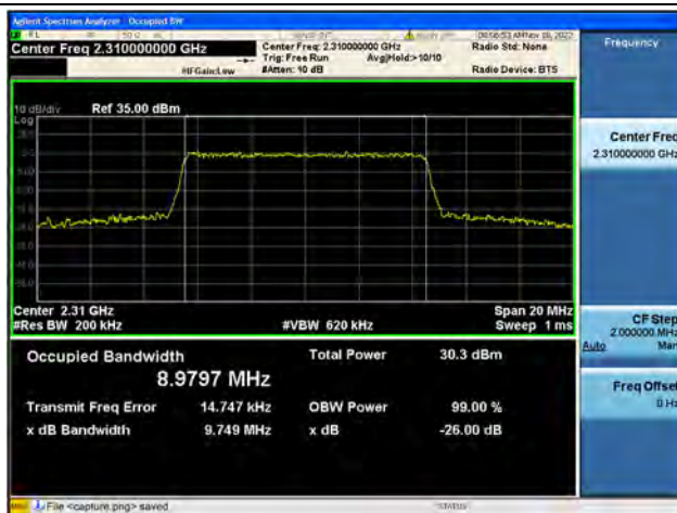
Band30 / 10MHz / 16QAM/ High CH
