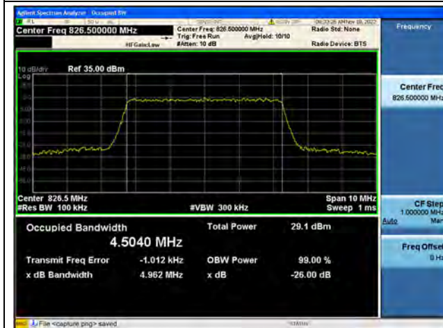
Band26Part22 / 5MHz / 64QAM/ Low CH
