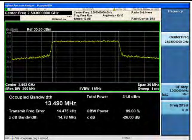
Band41 / 15MHz / QPSK/ Mid CH
