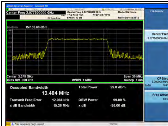
Band38 / 15MHz / QPSK/ Low CH
