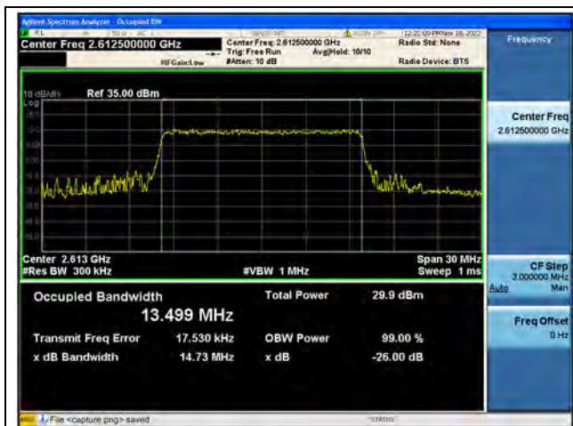
Band38 / 15MHz / QPSK/ High CH
