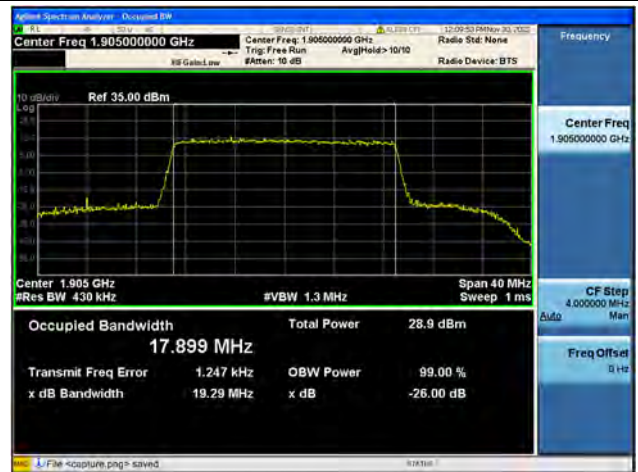
Band25 / 20MHz / QPSK/ High CH
