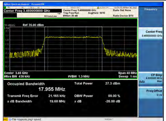
Band42 / 20MHz / 64QAM/ Low CH
