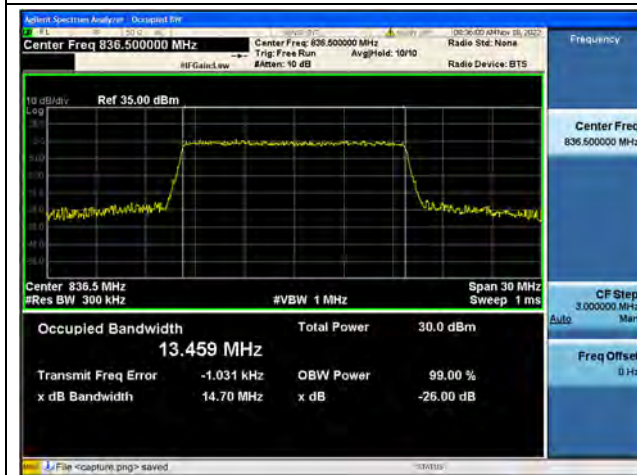
Band26Part22 / 15MHz / 16QAM/ Mid CH
