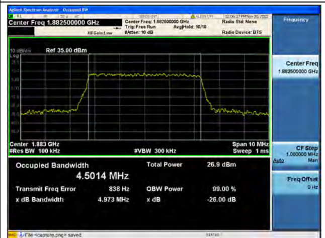
Band25 / 5MHz / 64QAM/ Mid CH
