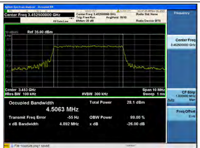
Band42 / 5MHz / 16QAM/ Low CH
