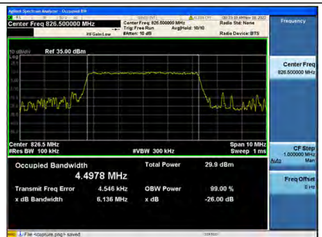
Band26Part22 / 5MHz / 16QAM/ Low CH
