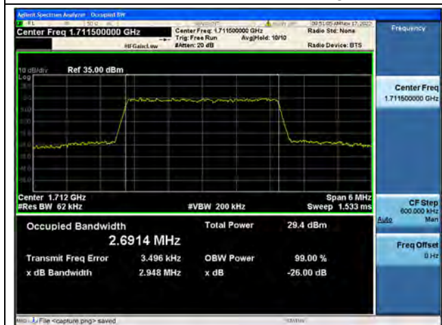
Band66 / 3MHz / 16QAM/ Low CH
