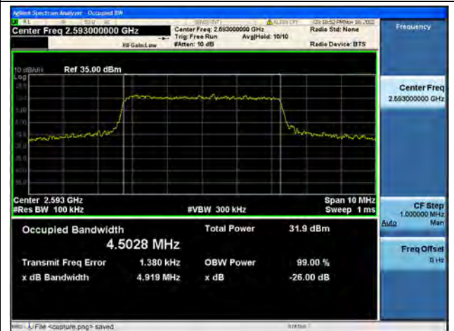
Band41 / 5MHz / QPSK/ Mid CH
