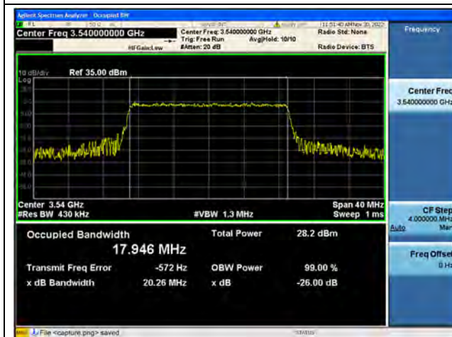
Band42 / 20MHz / 16QAM/ High CH
