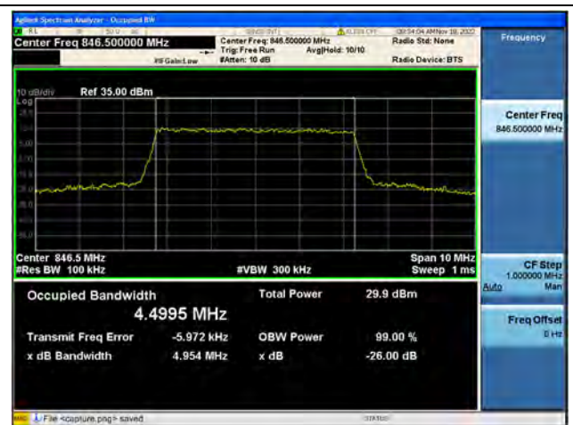
Band26Part22 / 5MHz / 16QAM/ High CH
