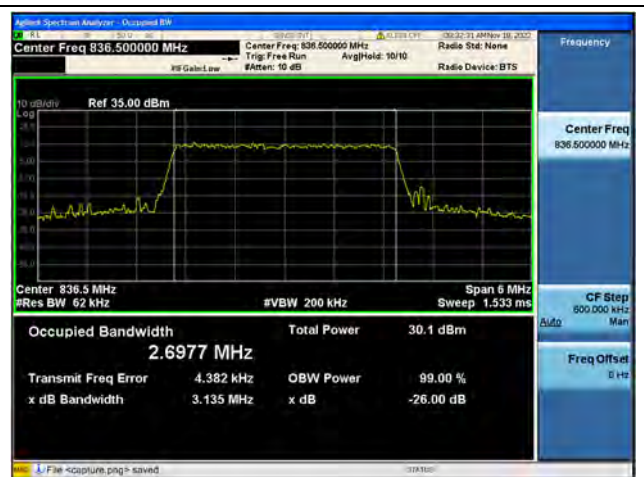
Band26Part22 / 3MHz / 16QAM/ Mid CH
