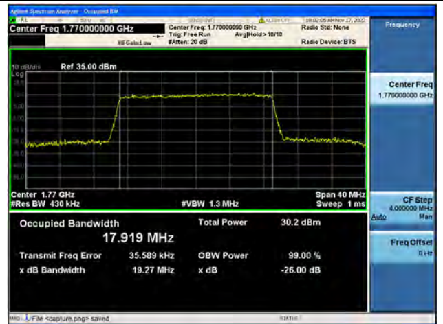
Band66 / 20MHz / QPSK/ High CH
