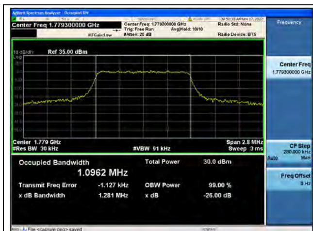
Band66 / 1.4MHz / QPSK/ High CH
