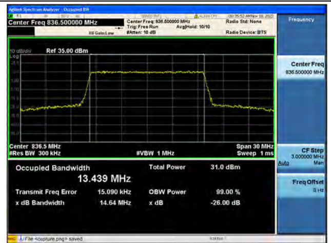
Band26Part22 / 15MHz / QPSK/ Mid CH
