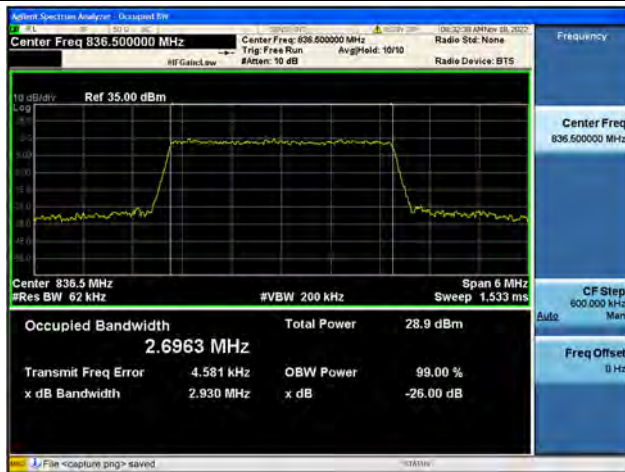
Band26Part22 / 3MHz / 64QAM/ Mid CH
