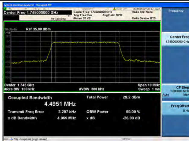
Band66 / 5MHz / 16QAM/ Mid CH
