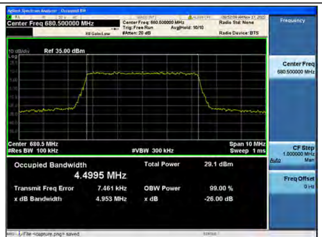
Band71 / 5MHz / 64QAM/ Mid CH
