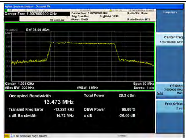
Band25 / 15MHz / 16QAM/ High CH
