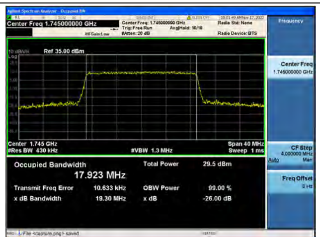
Band66 / 20MHz / 16QAM/ Mid CH
