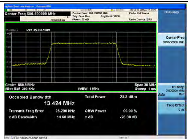
Band71 / 15MHz / 64QAM/ Mid CH
