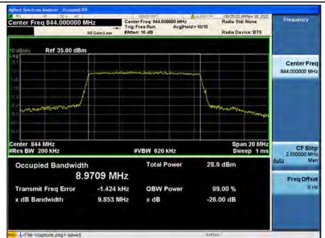
Band26Part22 / 10MHz / 64QAM/ High CH
