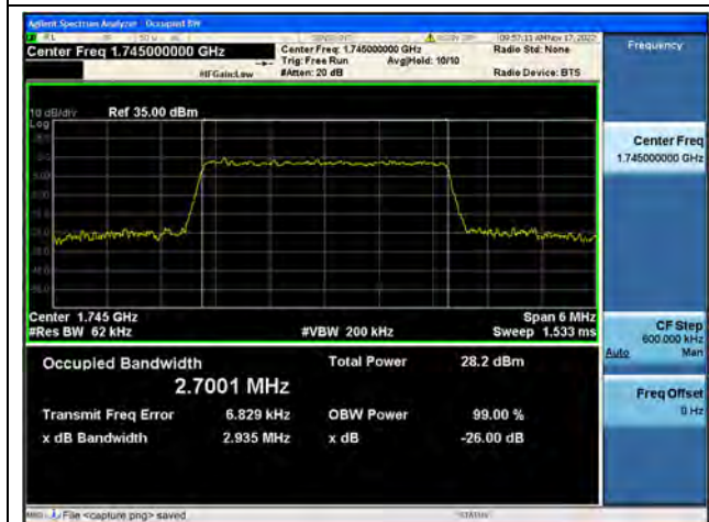
Band66 / 3MHz / 64QAM/ Mid CH
