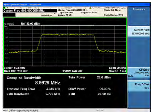
Band71 / 10MHz / 64QAM/ High CH
