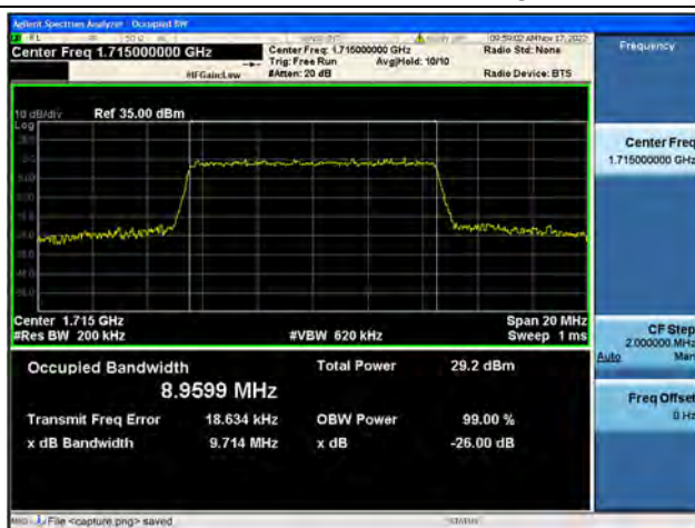
Band66 / 10MHz / 16QAM/ Low CH
