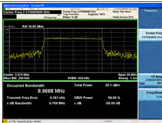
Band38 / 10MHz / 16QAM/ Low CH
