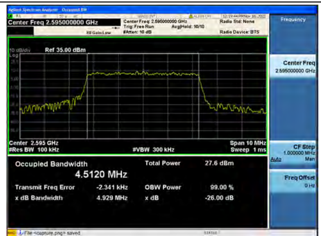
Band38 / 5MHz / 64QAM/ Mid CH
