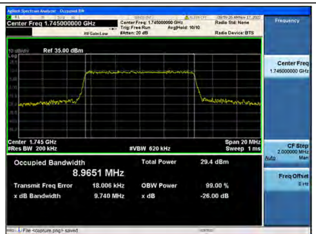
Band66 / 10MHz / 16QAM/ Mid CH
