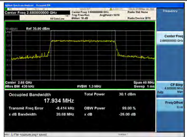
Band41 / 20MHz / QPSK/ High CH
