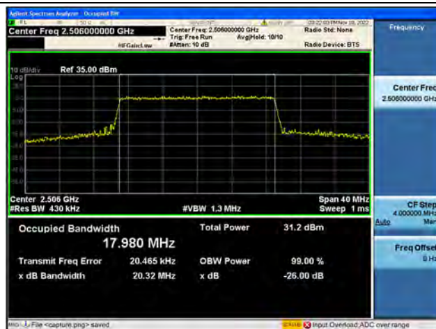
Band41 / 20MHz / 16QAM/ Low CH
