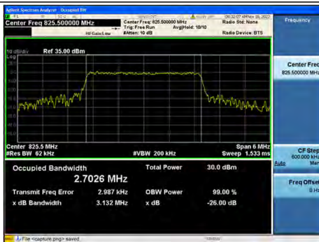
Band26Part22 / 3MHz / 16QAM / Low CH
