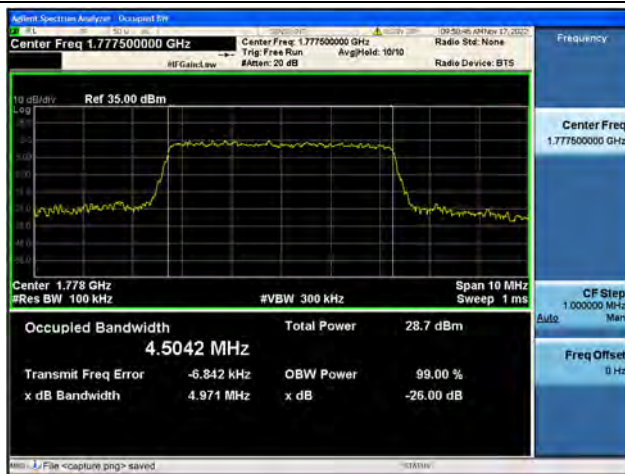
Band66 / 5MHz / 64QAM/ High CH
