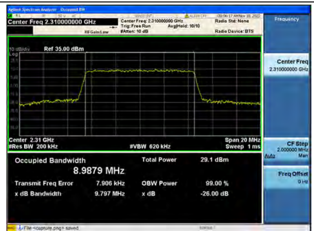
Band30 / 10MHz / 64QAM/ Low CH
