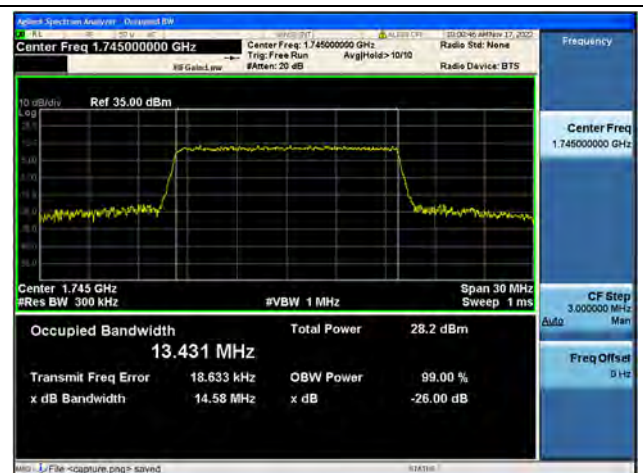
Band66 / 15MHz / 64QAM/ Mid CH
