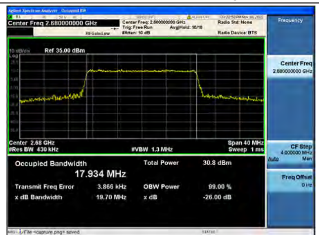
Band41 / 20MHz / 64QAM/ High CH
