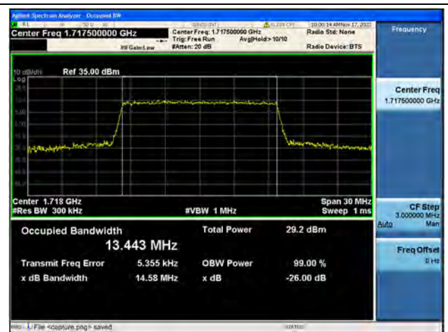
Band66 / 15MHz / 16QAM/ Low CH
