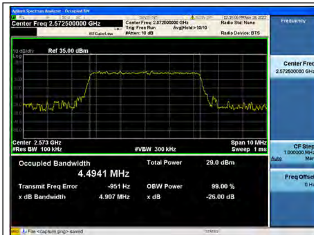
Band38 / 5MHz / QPSK/ Low CH
