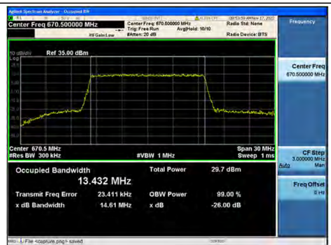
Band71 / 15MHz / 16QAM/ Low CH
