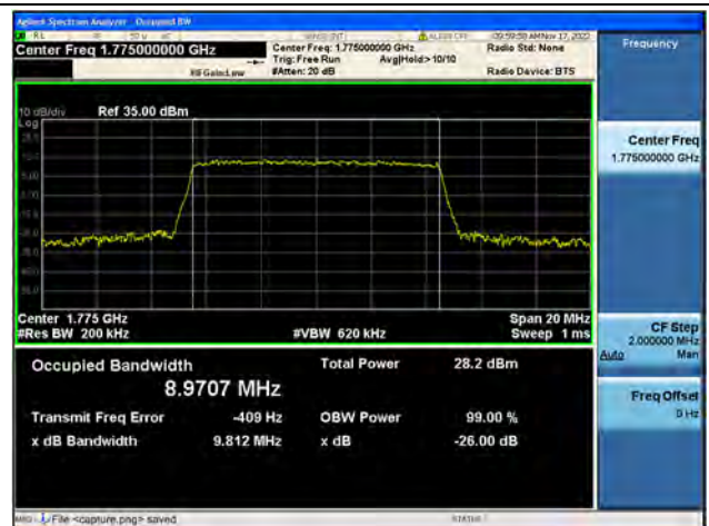
Band66 / 10MHz / 64QAM/ High CH
