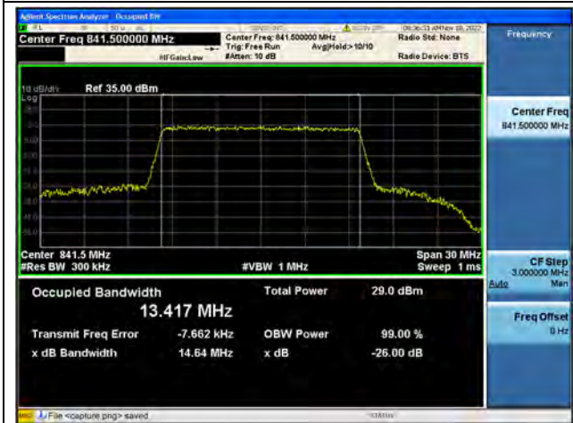
Band26Part22 / 15MHz / 64QAM/ High CH
