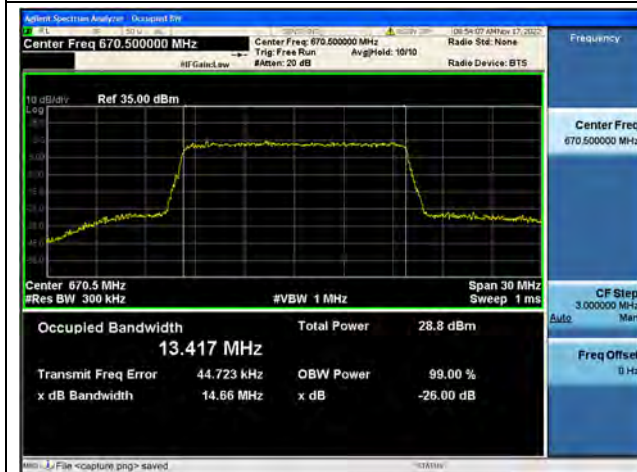
Band71 / 15MHz / 64QAM/ Low CH
