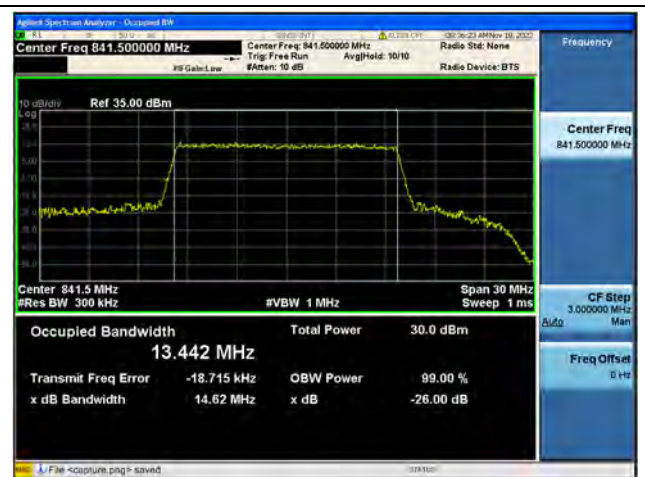
Band26Part22 / 15MHz / 16QAM/ High CH
