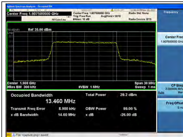
Band25 / 15MHz / QPSK/ High CH
