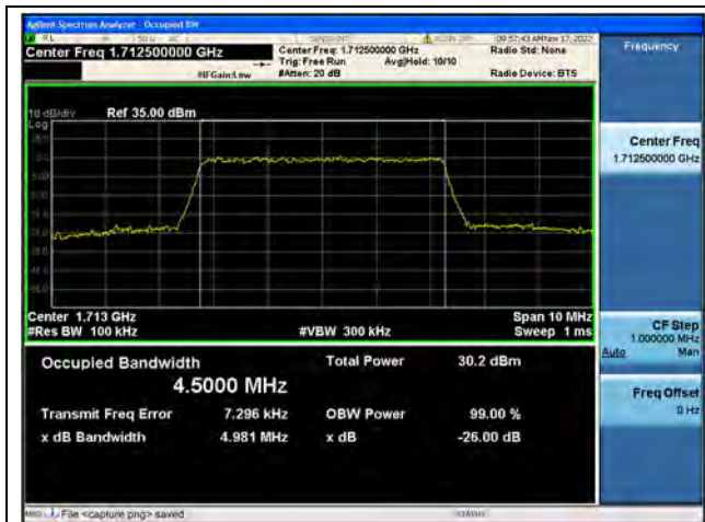
Band66 / 5MHz / QPSK/ Low CH
