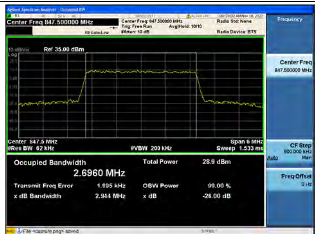
Band26Part22 / 3MHz / 64QAM/ High CH
