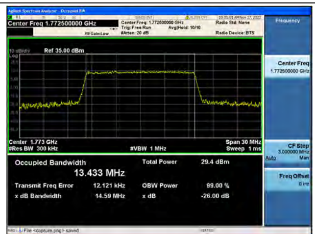
Band66 / 15MHz / 16QAM/ High CH
