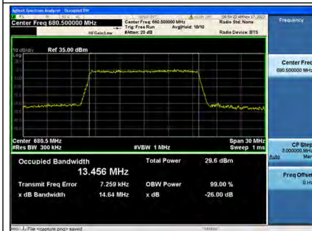
Band71 / 15MHz / 16QAM/ Mid CH
