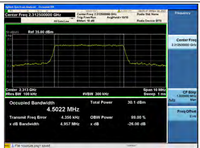
Band30 / 5MHz / 16QAM/ High CH
