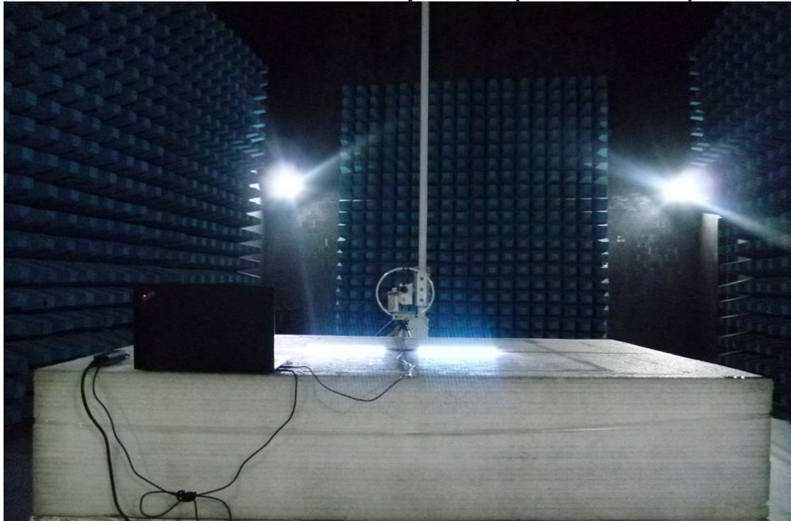
Radiated Emission Set up Photo (Below 1GHz)
