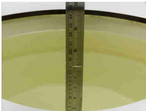
Fig 11.1 Photo of Liquid Height for Body SAR
