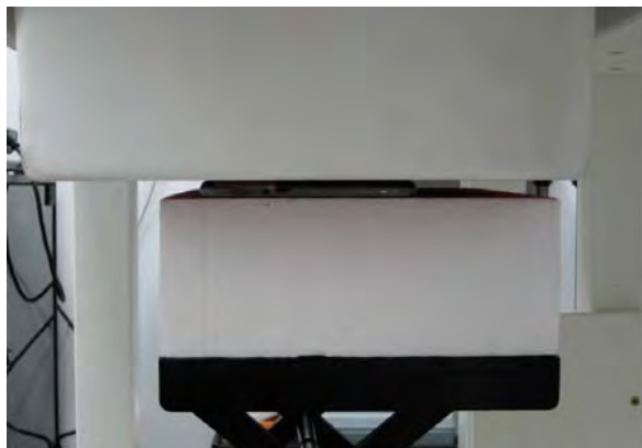
Fig.3 EUT Lap-held mode to flat phantom
