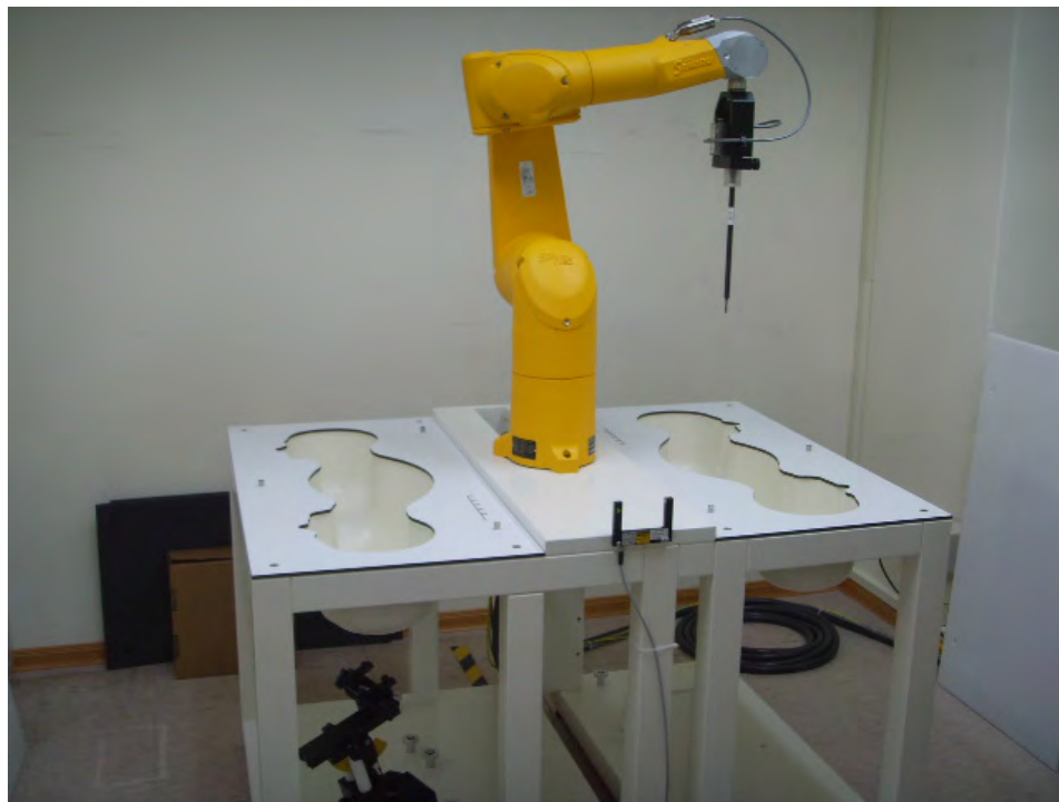
Fig.1 Photograph of the SAR measurement system
