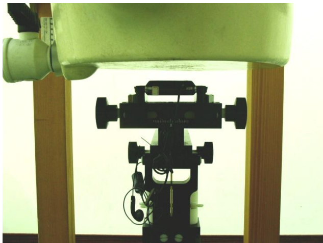
Bottom of the DUT with Phantom 1.5 cm Gap (DUT Slide Off)
