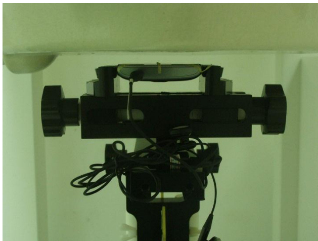
Front of the DUT with Phantom 1 cm Gap (DUT with Earphone)
