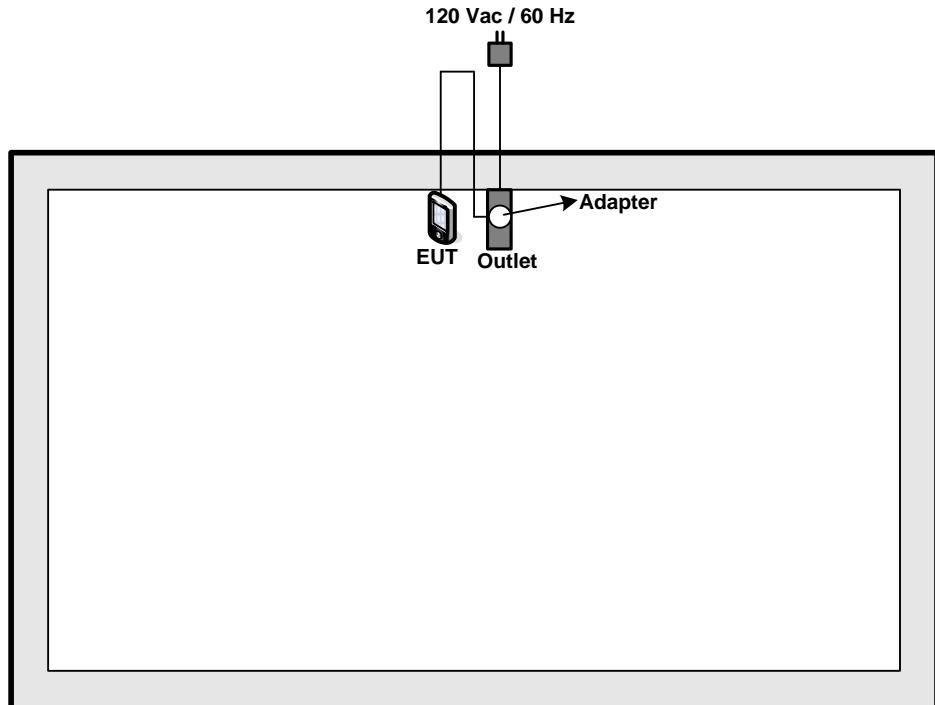
For radiated emissions 30MHz~1GHz
