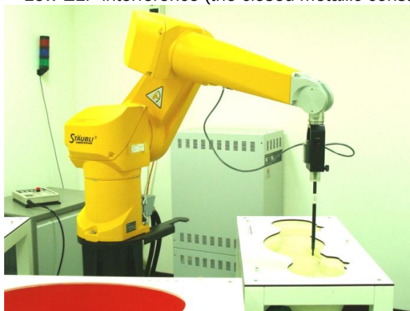
Fig 5.5 Photo of DASY4
