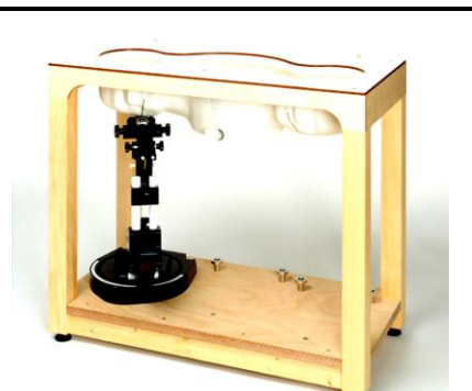
Fig 5.9 Photo of SAM Phantom
