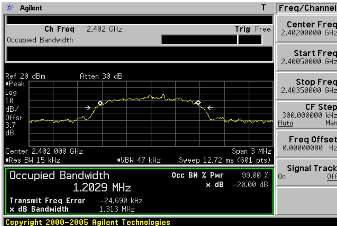
**20dB Bandwidth Test Data CH-Mid**
