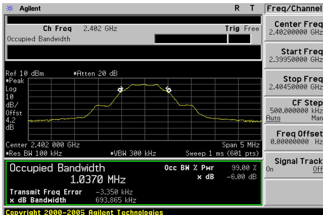
**6dB Band Width Test Data CH-Mid**
