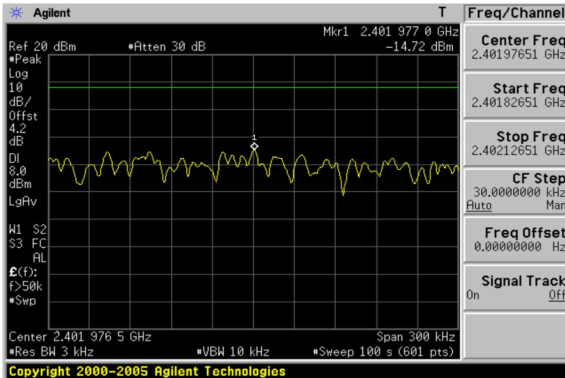
**Power Spectral Density Test Plot (CH-Mid)**
