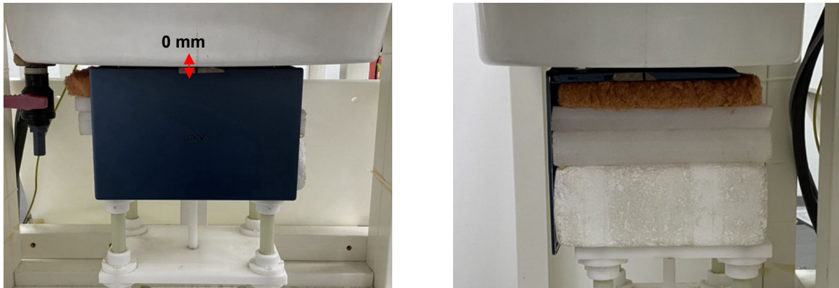
Fig.3 EUT Bottom side to flat phantom
