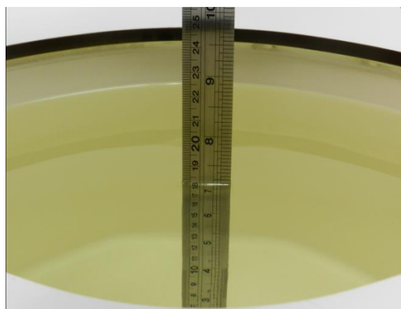
Fig 10.2 Photo of Liquid Height for Body SAR
