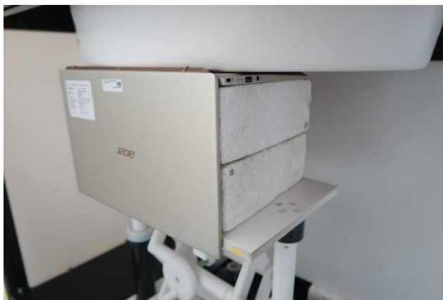
Bottom of Laptop, Test Separation 0 mm
