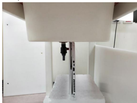
Fig.5 EUT Bottom side (TB mode) to flat phantom
