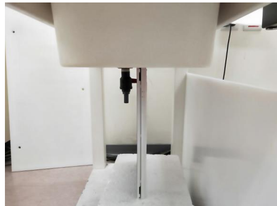
Fig.7 EUT Left side to flat phantom
