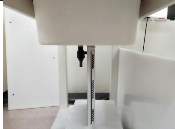
Fig.6 EUT Right side to flat phantom
