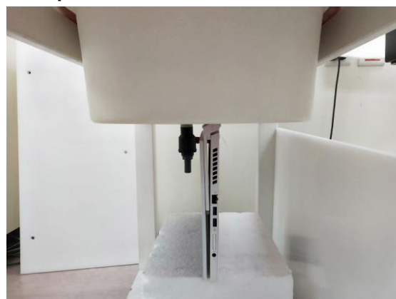
Fig.4 EUT Top side to flat phantom
