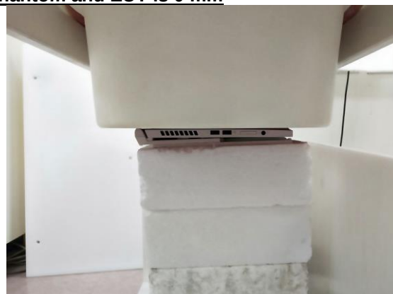
Fig.3 EUT Back side to flat phantom
