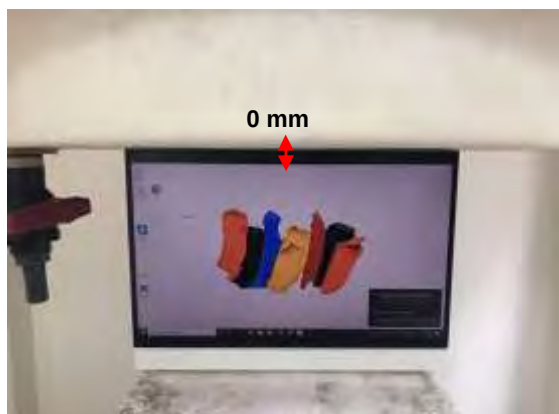
Fig.5 EUT Bottom side to flat phantom
