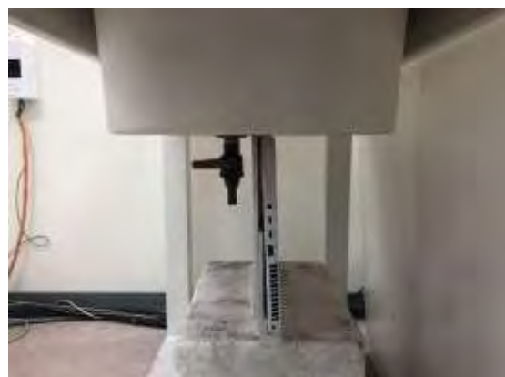
Fig.5 EUT Bottom side to flat phantom
