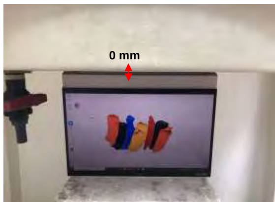
Fig.4 EUT Top side to flat phantom
