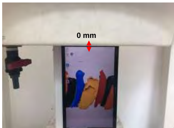
Fig.6 EUT Right side to flat phantom
