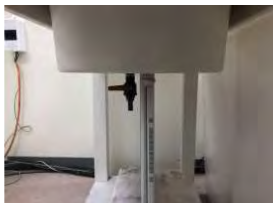
Fig.7 EUT Left side to flat phantom
