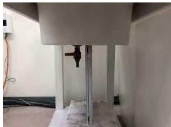
Fig.6 EUT Right side to flat phantom
