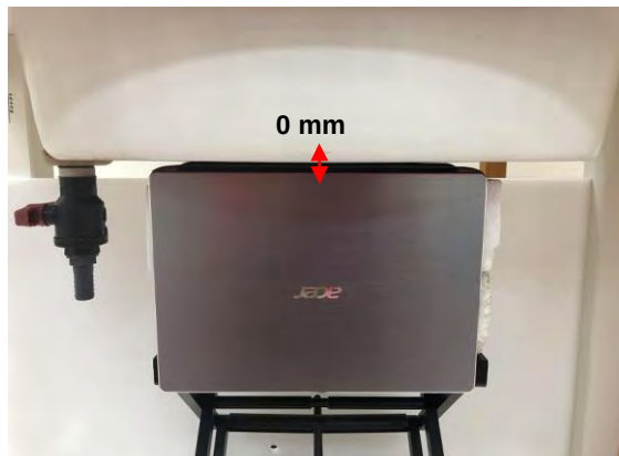
Fig.3 EUT Bottom side to flat phantom
