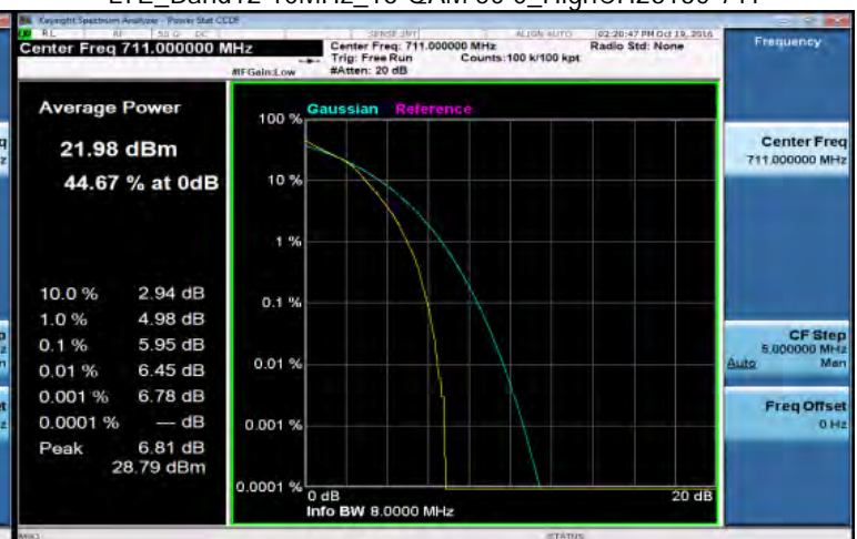
LTE_Band12 10MHz_16-QAM 50 0_HighCH23130-711
