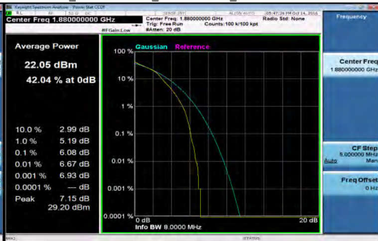
LTE_Band2 10MHz_16-QAM 50 0_HighCH19150-1905
