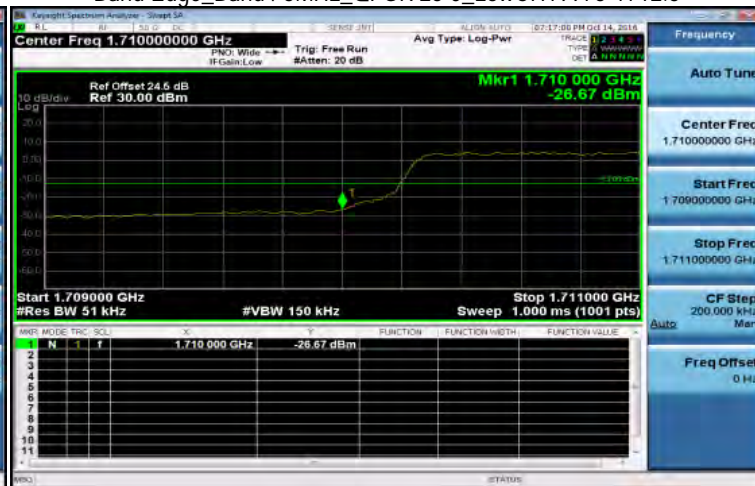
Band Edge_Band4 5MHz_QPSK 25 0_LowCH19975-1712.5
