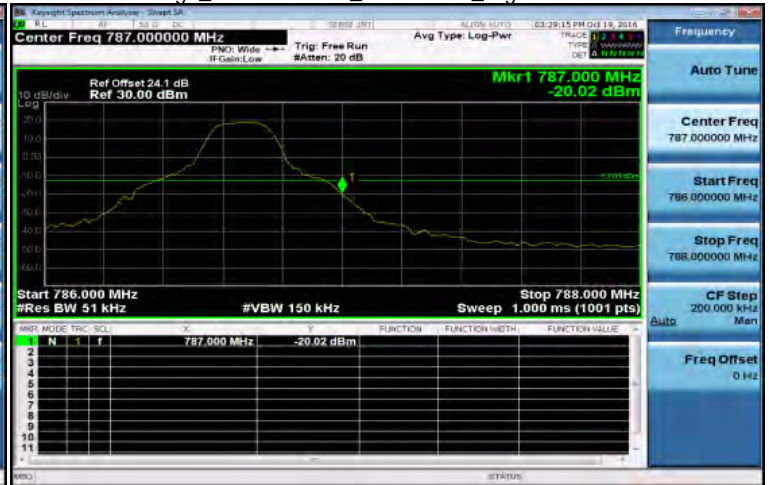
Band Edge_Band13 5MHz_QPSK 1 24_HighCH23255-784.5
