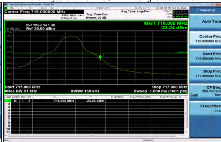
Band Edge_Band17 5MHz_QPSK 1 24_HighCH23825-713.5
