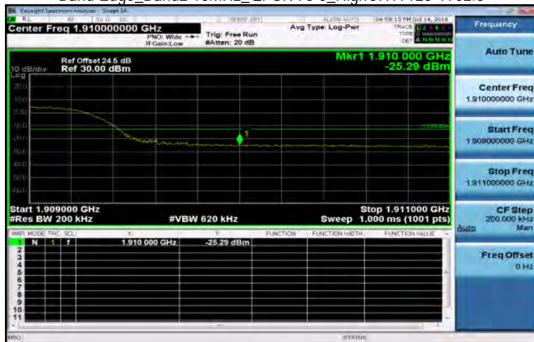
Band Edge_Band2 15MHz_QPSK 75 0_HighCH19125-1902.5
