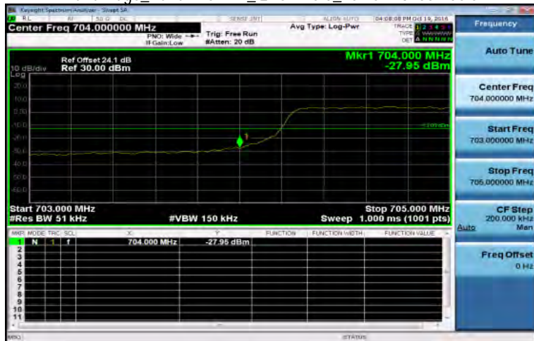
Band Edge_Band17 5MHz_QPSK 25 0_LowCH23755-706.5
