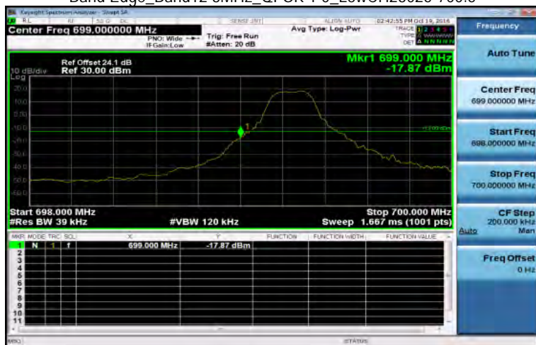
Band Edge_Band12 3MHz_QPSK 1 0_LowCH23025-700.5
