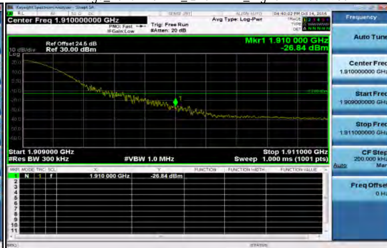
Band Edge_Band2 20MHz_QPSK 1 99_HighCH19100-1900
