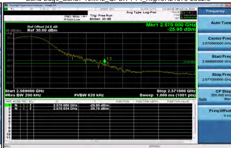
Band Edge_Band7 15MHz_QPSK 1 74_HighCH21375-2562.5
