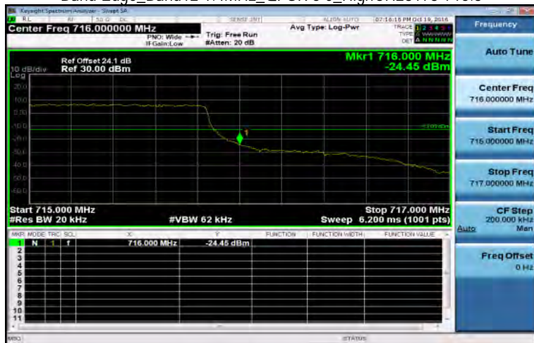
Band Edge_Band12 1.4MHz_QPSK 6 0_HighCH23173-715.3
