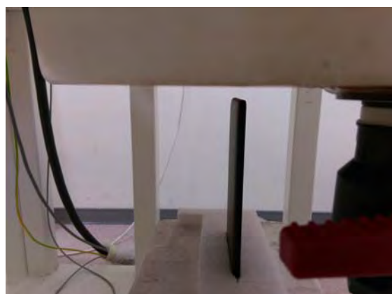
Fig.7 EUT Top side (13mm) to flat phantom
