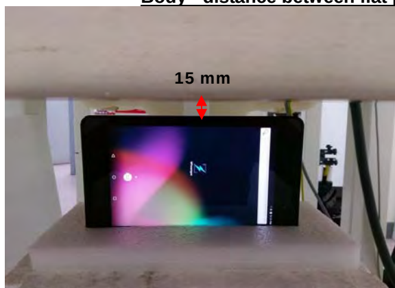
Fig.9 EUT Left side (15mm) to flat phantom
