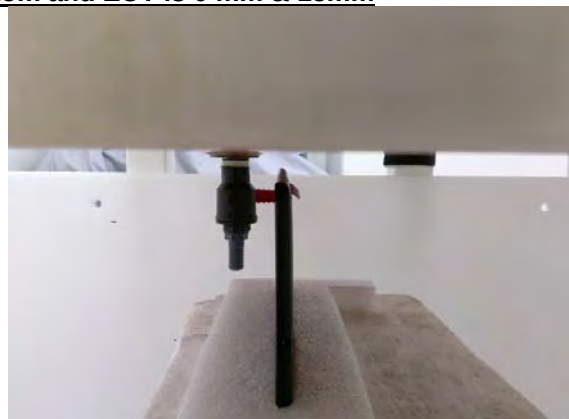
Fig.9 EUT Left side (15mm) to flat phantom
