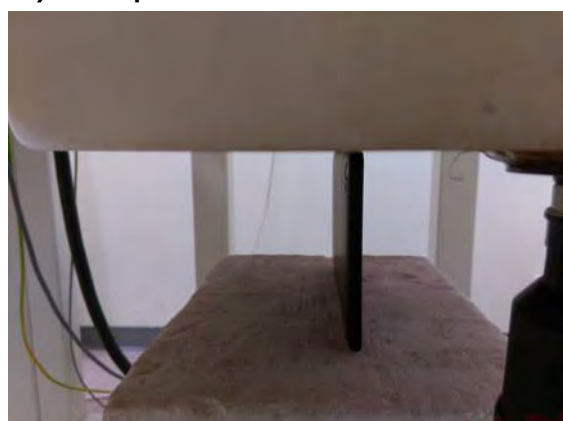
Fig.5 EUT Right side to flat phantom
