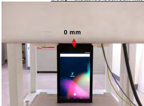
Fig.6 EUT Top side to flat phantom
