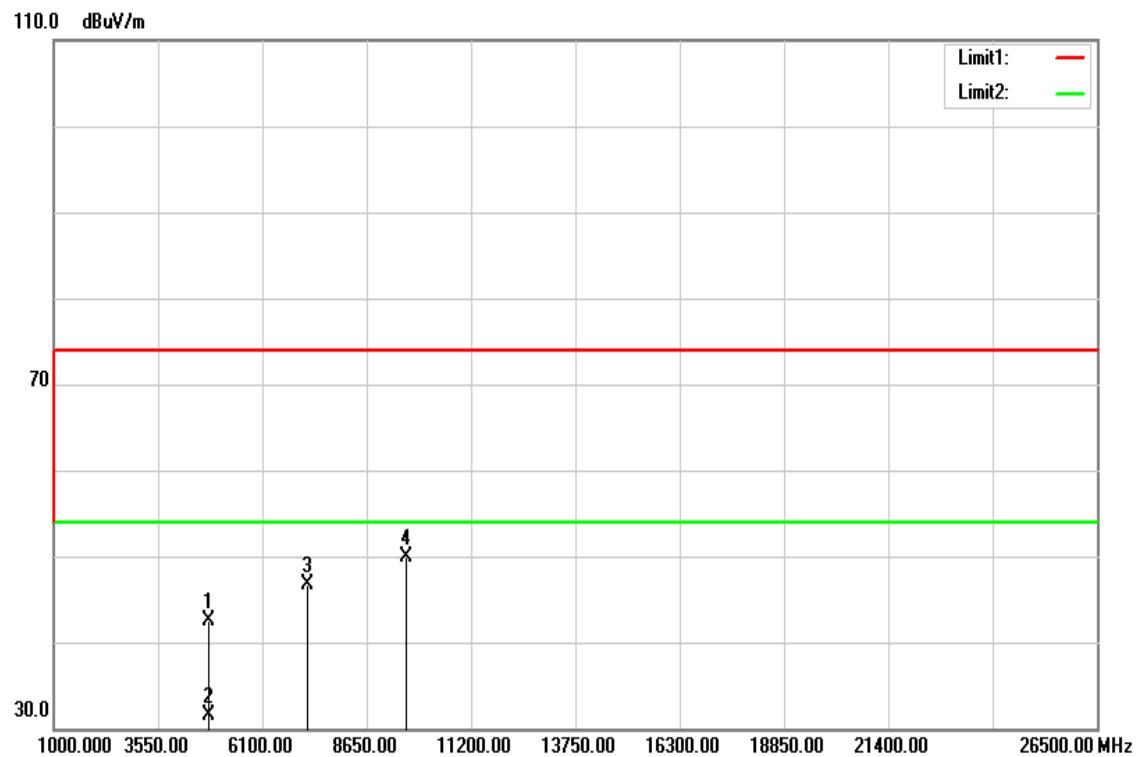
**Above 1 GHz****Operation Mode:** TX / GFSK / DH5 / CH Low**Test Date:** June 1, 2016**Temperature:** 27°C**Tested by:** Dennis Li**Humidity:** 53 % RH**Polarity:** Ver. / Hor.
