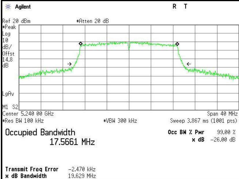
**IEEE 802.11n HT 20 MHz mode / 5260~ 5320MHz****26dB Bandwidth (CH Low)**
