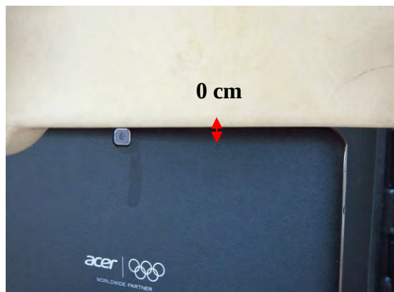
Fig.5 EUT Secondary Landscape mode to flat phantom
