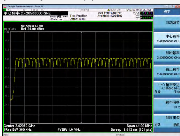
GFSK 2.4 GHz ~ 2.4415 GHz
