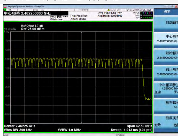
GFSK 2.4415 GHz ~ 2.4835 GHz
