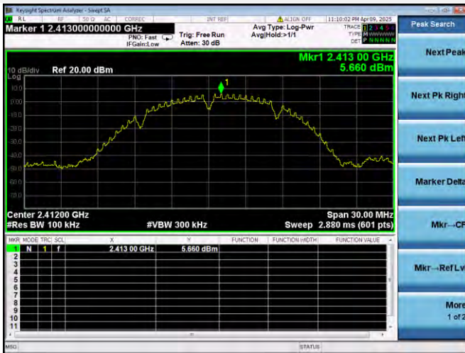
802.11b LOW CHANNEL, CARRIER LEVEL
