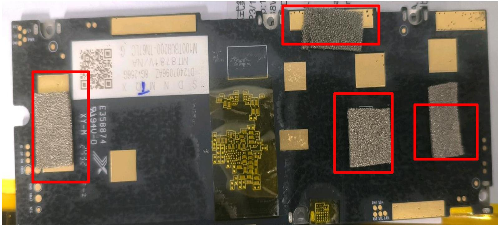
1. On the back of the main board, the conductive sponge at the corresponding position of the red frame is grounded to the radium carving position of the metal back shell;
