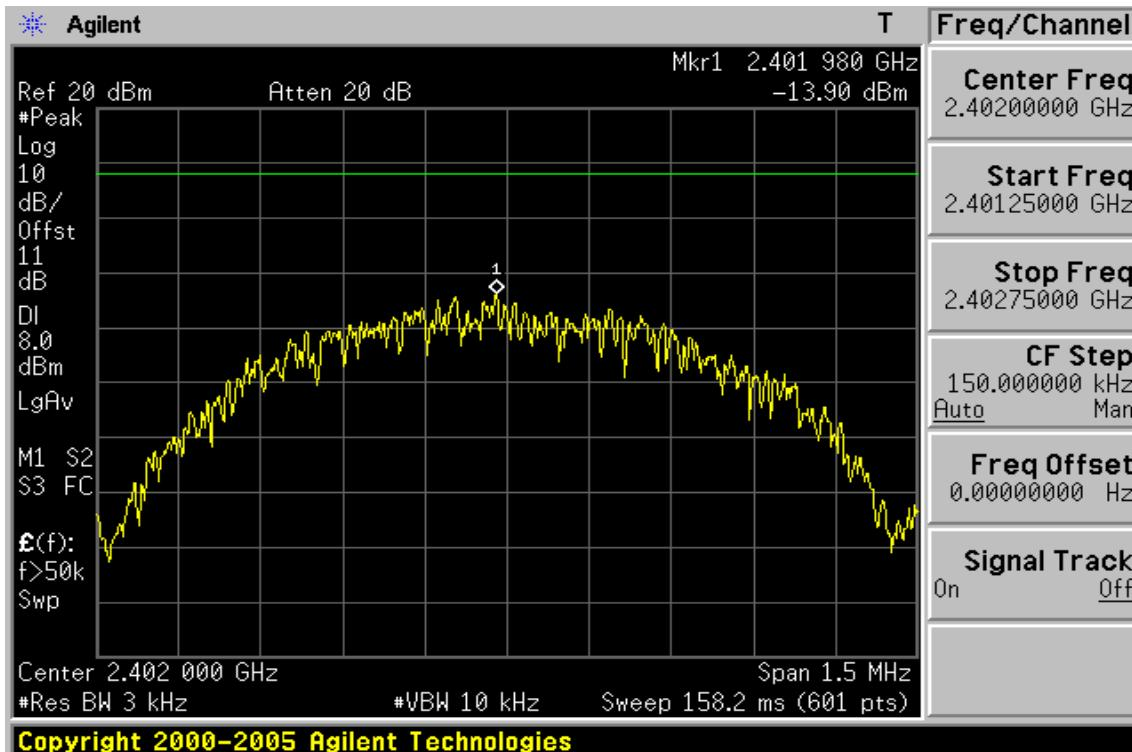
**Power Spectral Density Test Plot (CH-Mid)**
