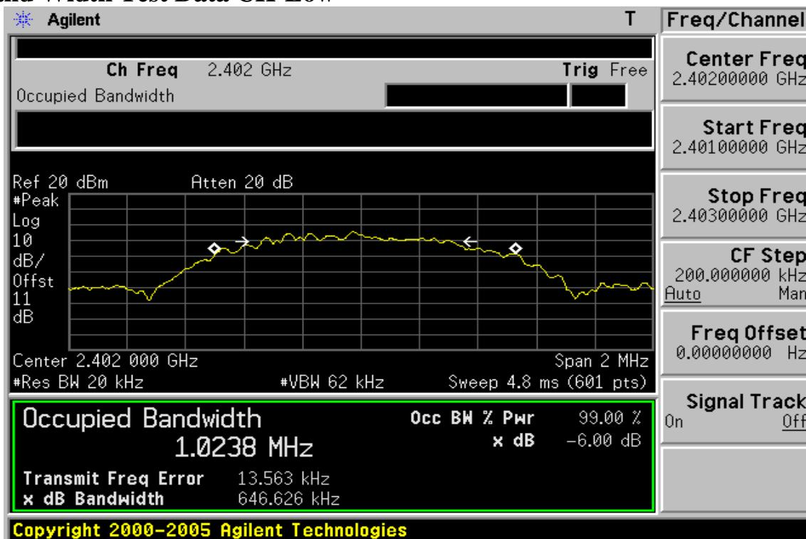
**99% Band Width Test Data CH-Mid**
