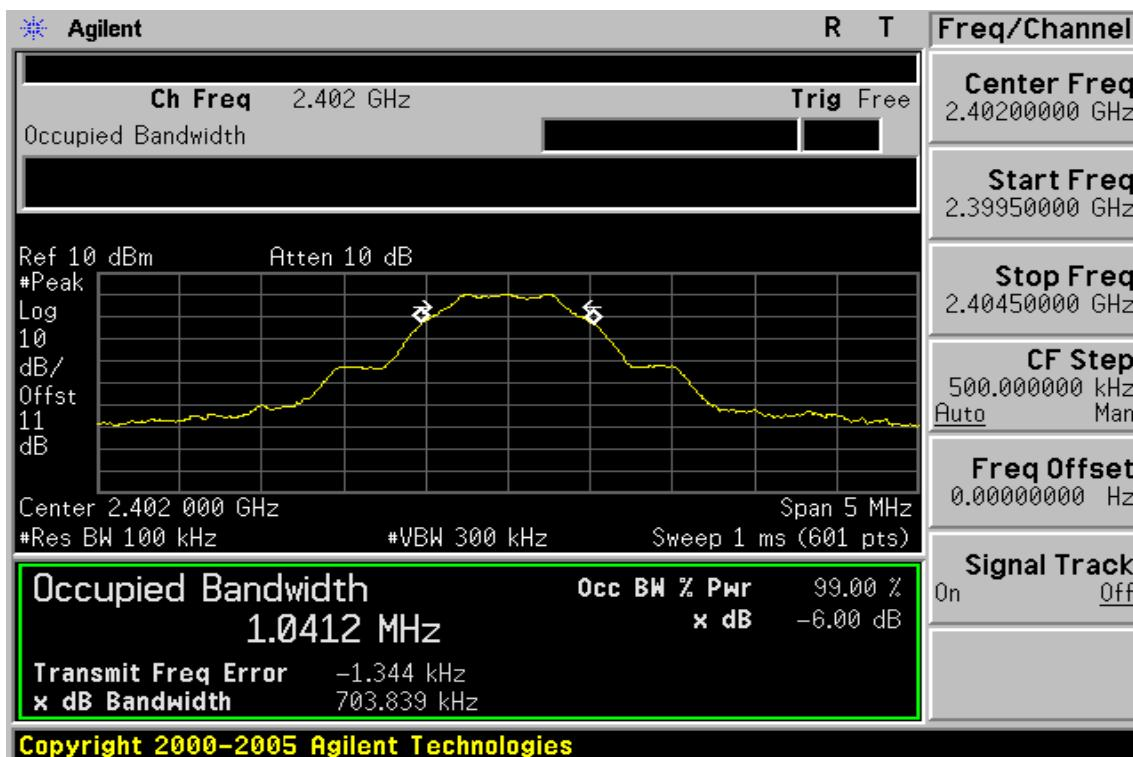
**6dB Band Width Test Data CH-Mid**
