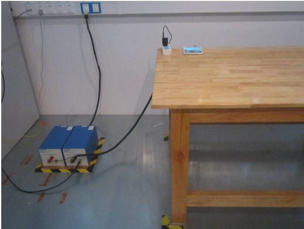
Conducted Emissions Test Setup Front View(Adapter2)
