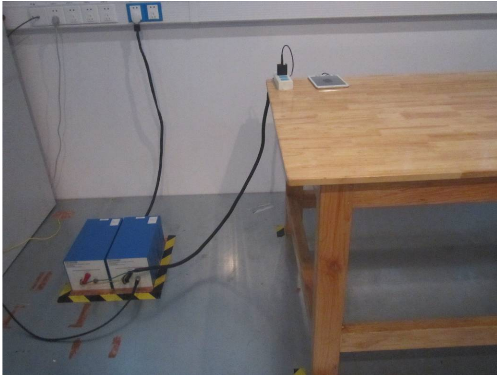
Conducted Emissions Test Setup Front View(Adapter1)
