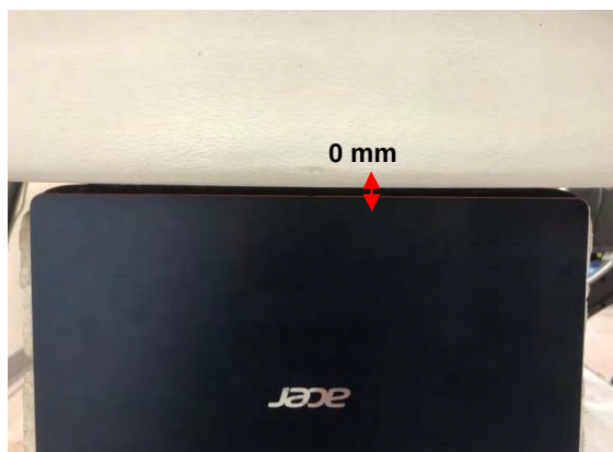
Fig.3 EUT Bottom side to flat phantom
