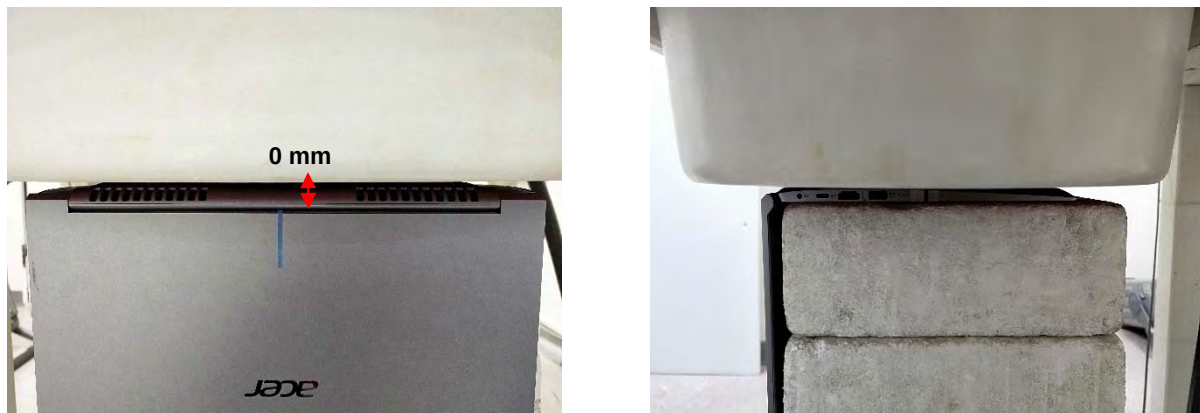
Fig.3 EUT Bottom side to flat phantom
