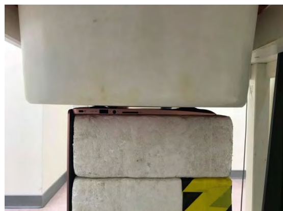
Fig.3 EUT Bottom side to flat phantom
