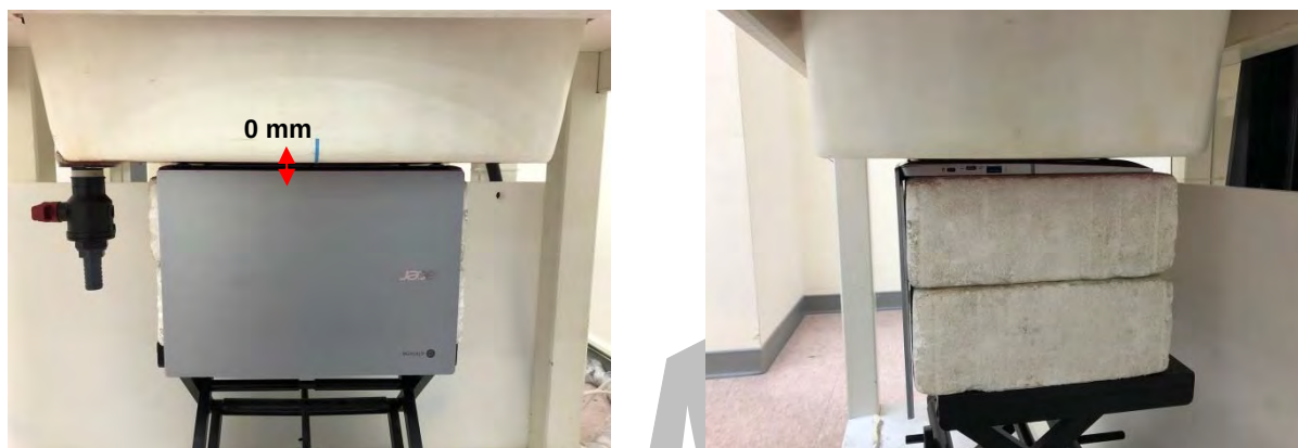
Fig.3 EUT Bottom side to flat phantom
