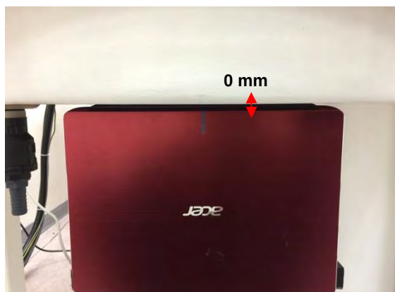
Fig.3 EUT Bottom side to flat phantom
