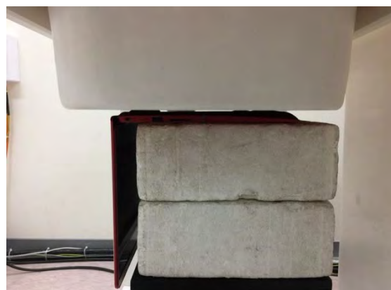
Fig.3 EUT Bottom side to flat phantom
