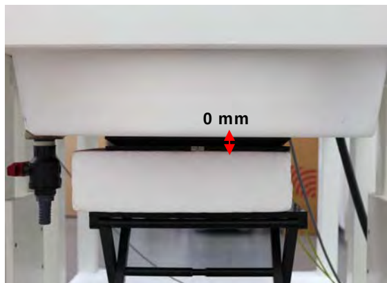
Fig.3 EUT Back side to flat phantom
