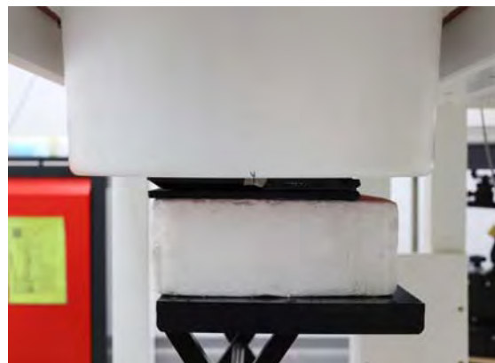
Fig.3 EUT Back side to flat phantom
