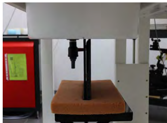
Fig.4 EUT Top side to flat phantom
