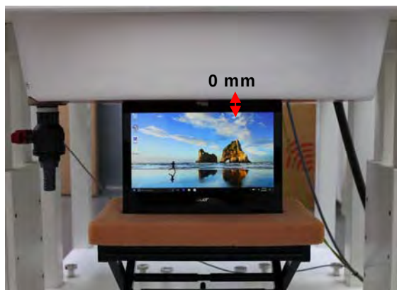
Fig.4 EUT Top side to flat phantom
