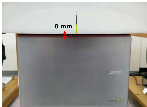
Fig.3 EUT Bottom side to flat phantom
