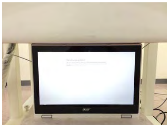
Fig.4 EUT Top side to flat phantom
