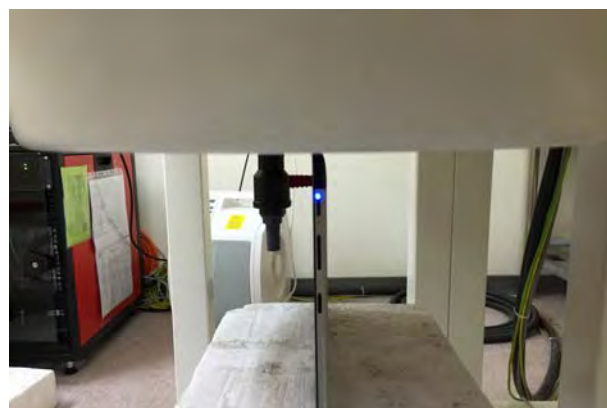
Fig.4 EUT Top side to flat phantom
