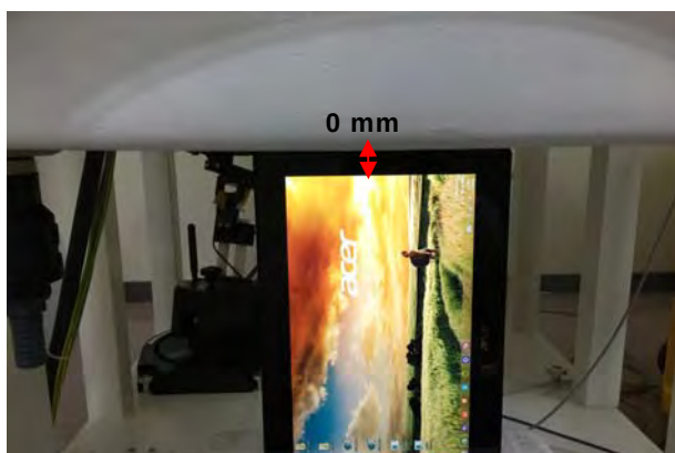
Fig.6 EUT Right side to flat phantom
