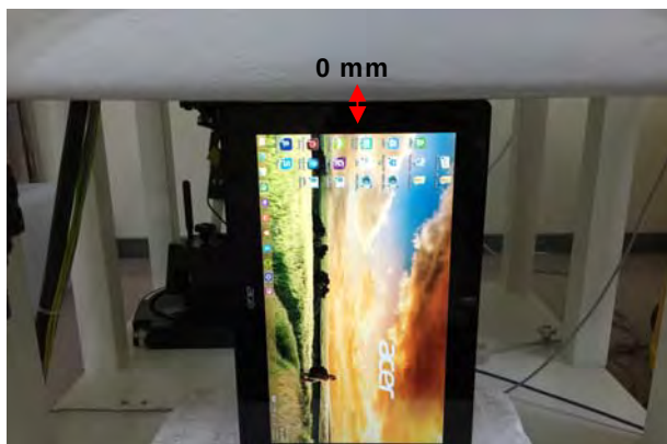
Fig.5 EUT Left side to flat phantom
