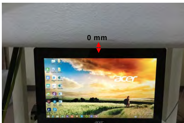
Fig.4 EUT Top side to flat phantom
