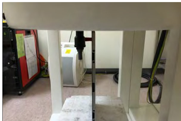
Fig.6 EUT Right side to flat phantom
