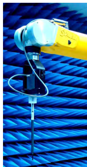
Figure 5. Probe setup on robot
