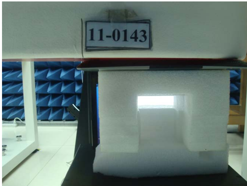
Figure 1. Body SAR Test Setup (Bottom Close Body)_Chain0
