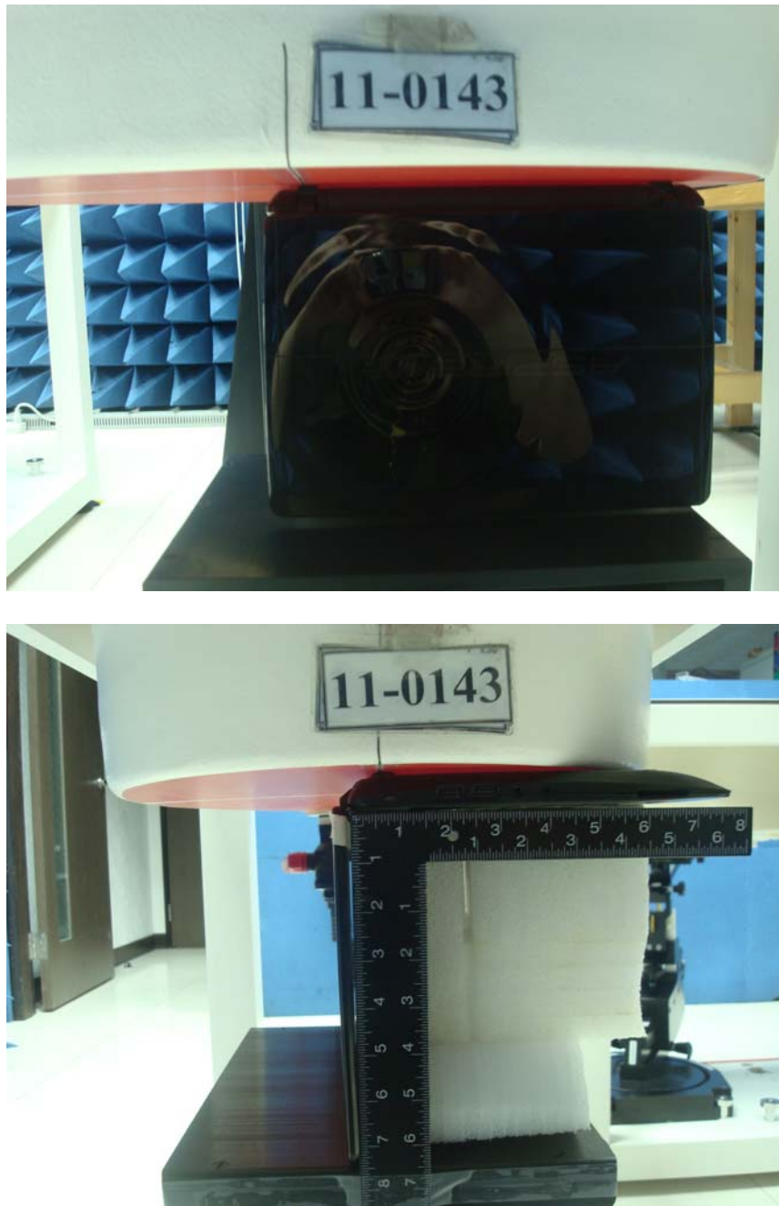
Figure 2. Body SAR Test Setup (Bottom Close Body)_Chain1
