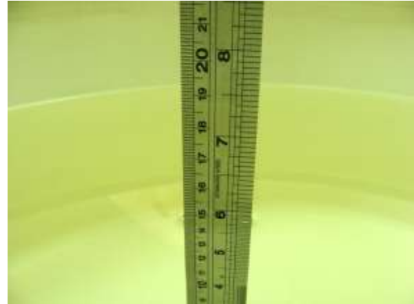
Fig 6.2 Photo of Liquid Height for Body SAR
