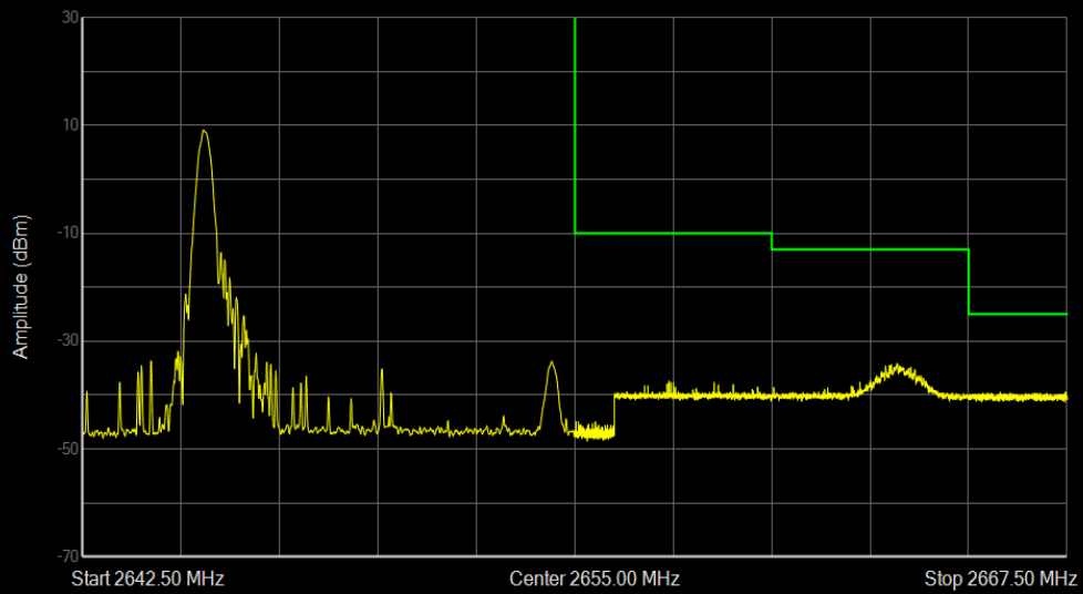
Band41 QPSK BW=10MHz Channel=41190 RB Size=1 Position=#0
