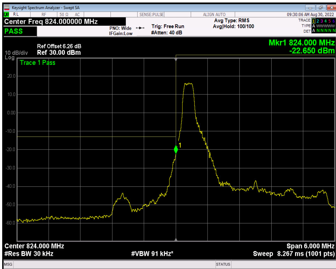
Band5 QPSK BW=3MHz Channel=20415 RB Size=1 Position=#Max
