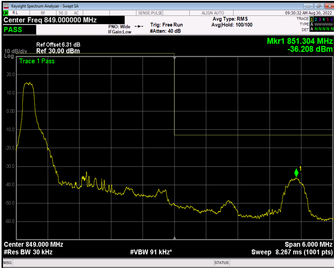
Band5 QAM16 BW=3MHz Channel=20635 RB Size=1 Position=#Max
