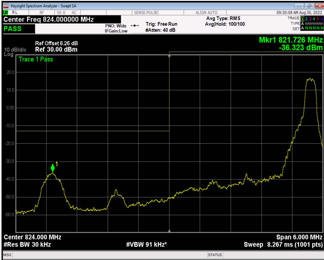
Band5 QPSK BW=3MHz Channel=20415 RB Size=15 Position=#0
