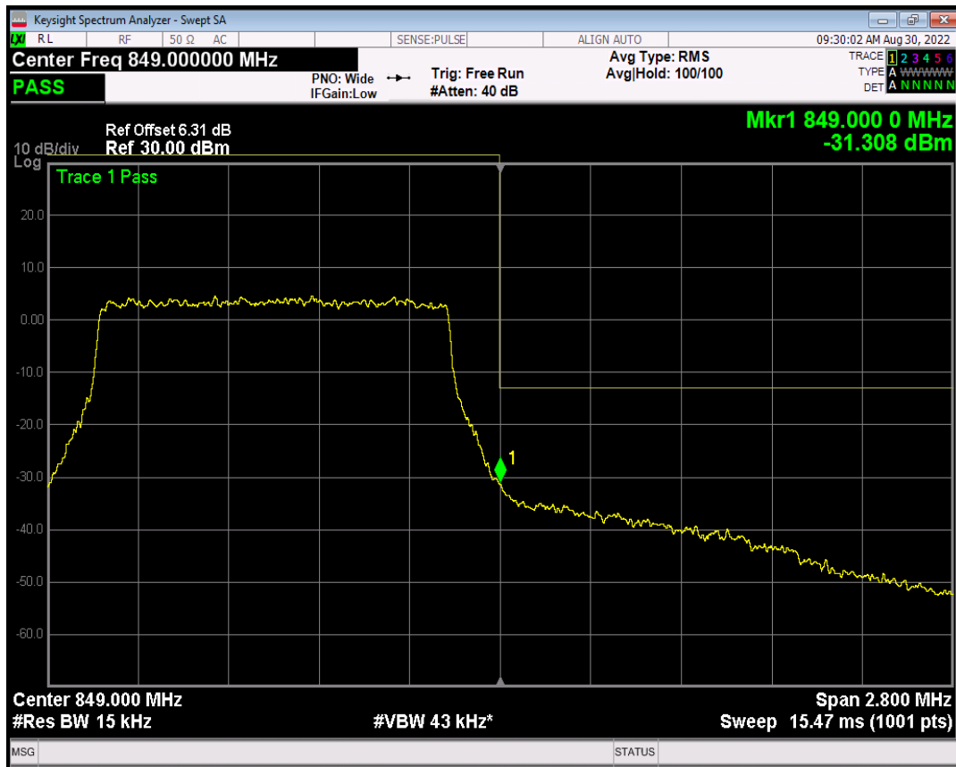
Band5 QPSK BW=3MHz Channel=20415 RB Size=1 Position=#0
