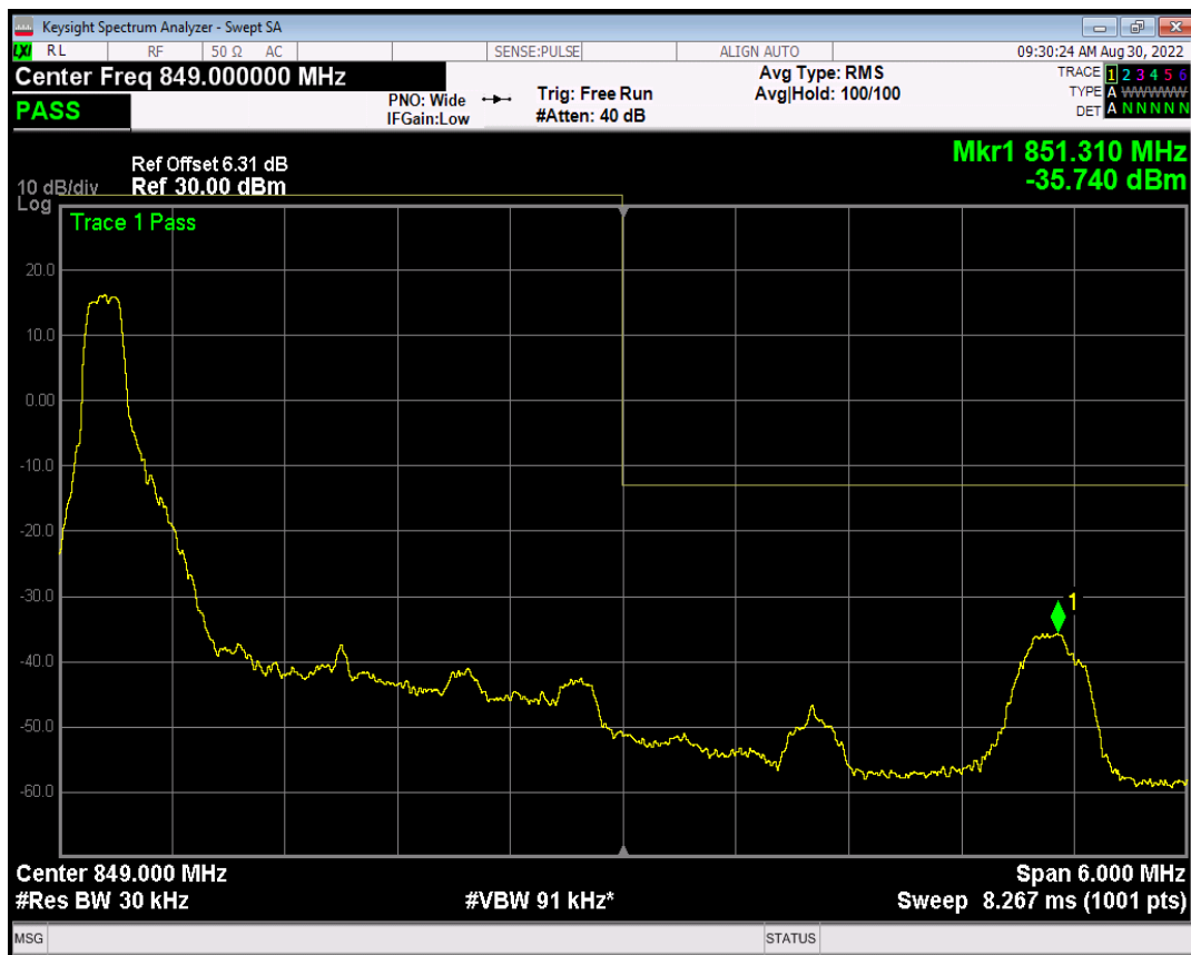
Band5 QPSK BW=3MHz Channel=20635 RB Size=1 Position=#Max
