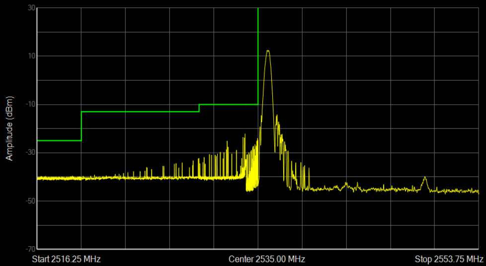
Band41 QPSK BW=15MHz Channel=40115 RB Size=1 Position=#0
