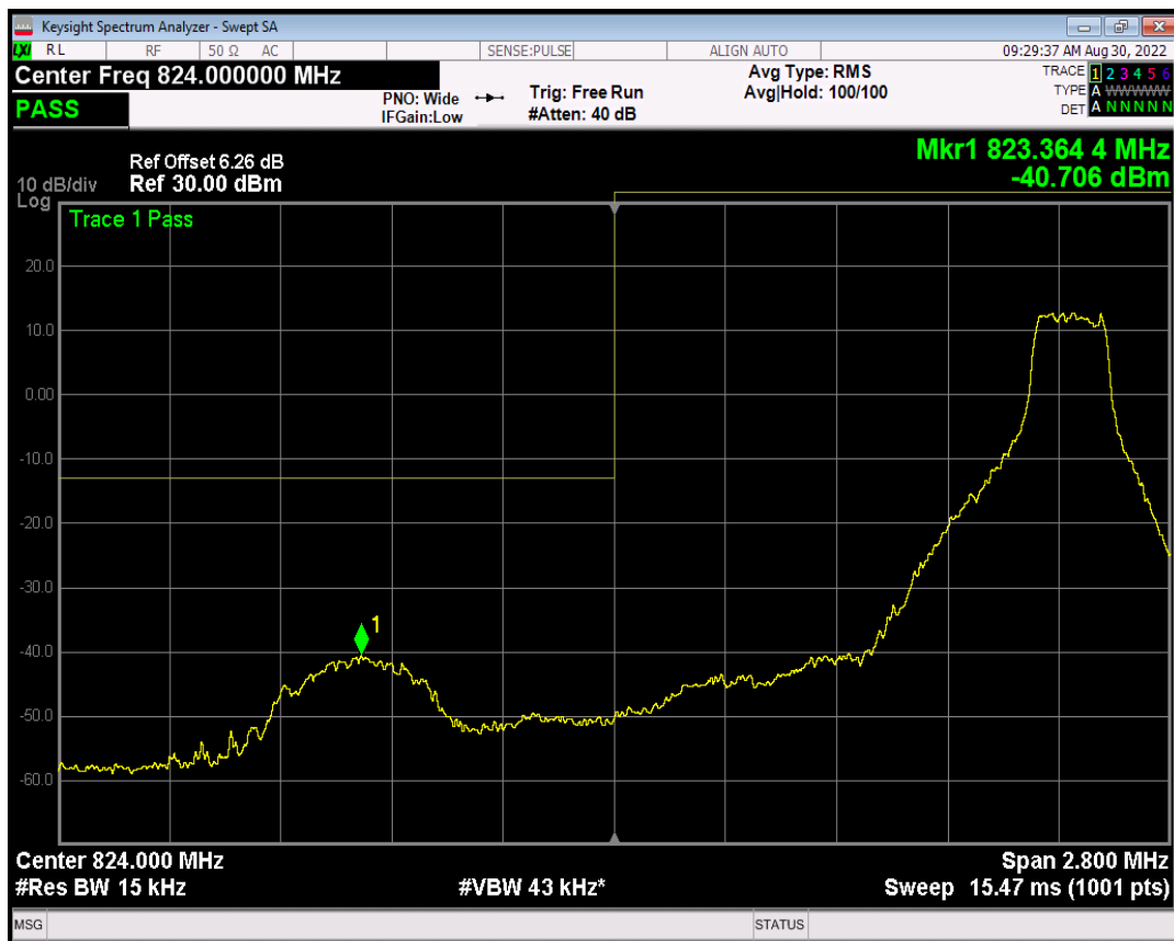
Band5 QAM16 BW=1.4MHz Channel=20407 RB Size=6 Position=#0
