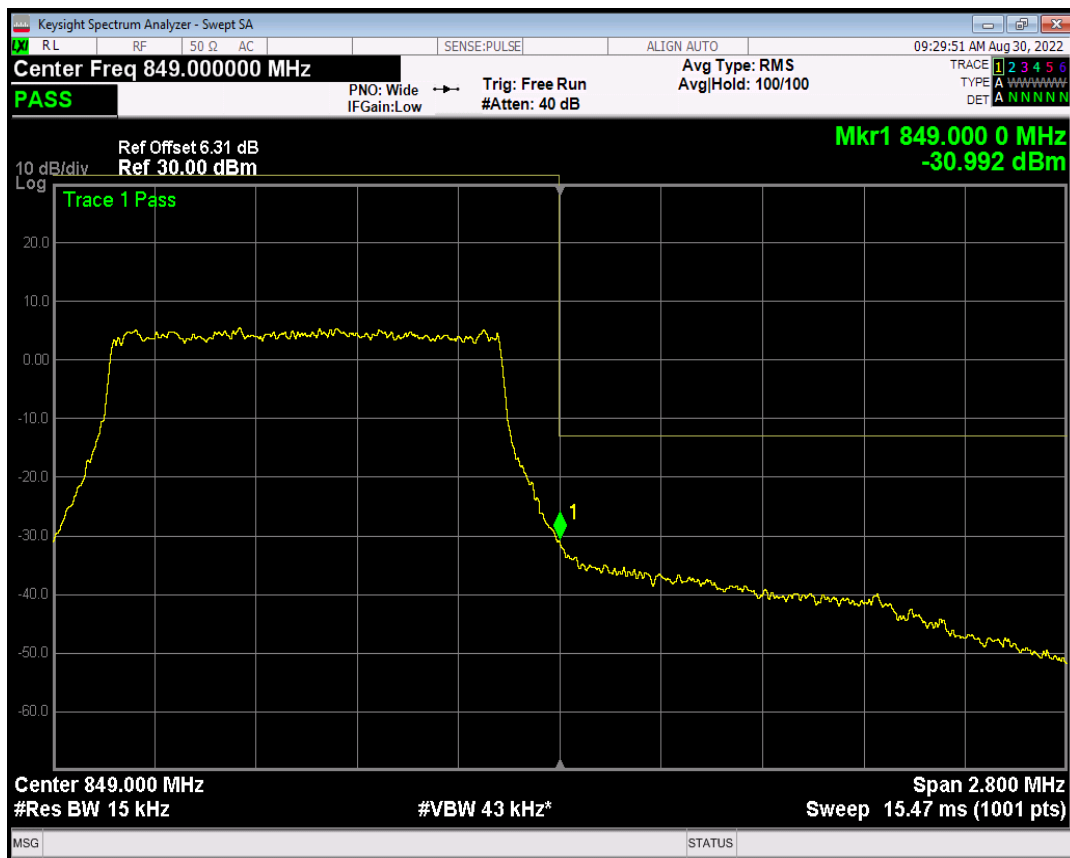
Band5 QAM16 BW=1.4MHz Channel=20643 RB Size=1 Position=#0
