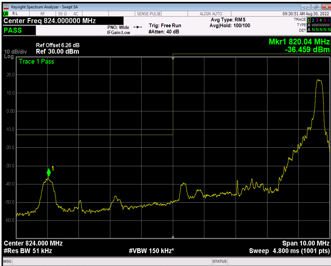
Band5 QAM16 BW=5MHz Channel=20425 RB Size=25 Position=#0
