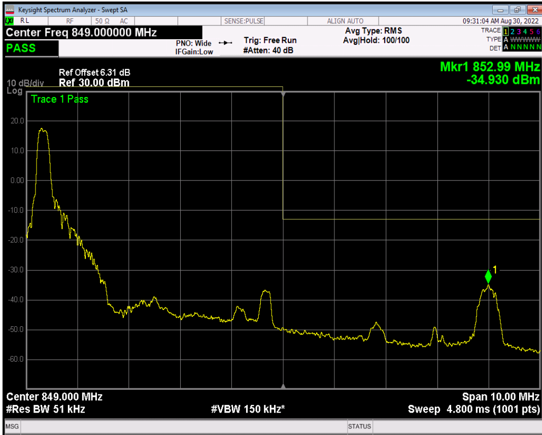
Band5 QAM16 BW=5MHz Channel=20625 RB Size=1 Position=#Max
