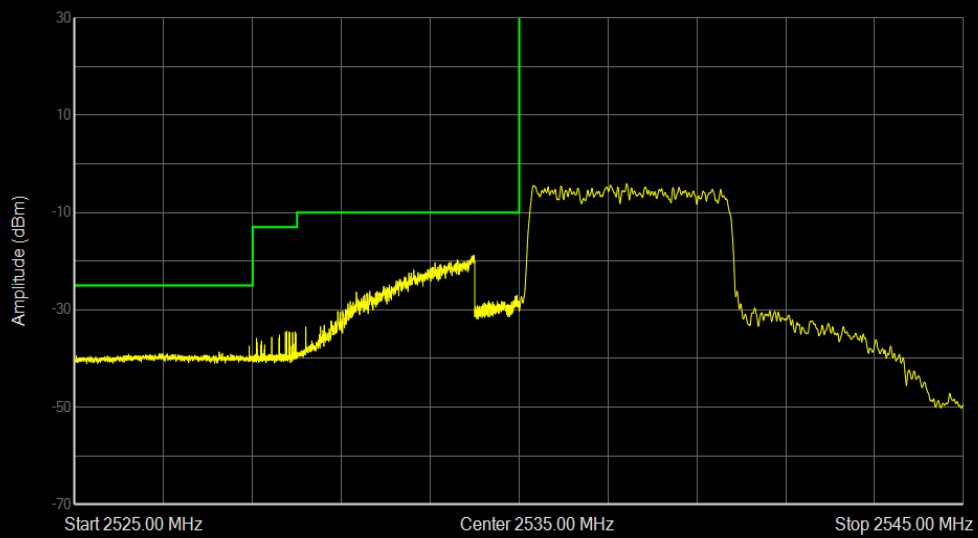
Band41 QPSK BW=5MHz Channel=40065 RB Size=25 Position=#0
