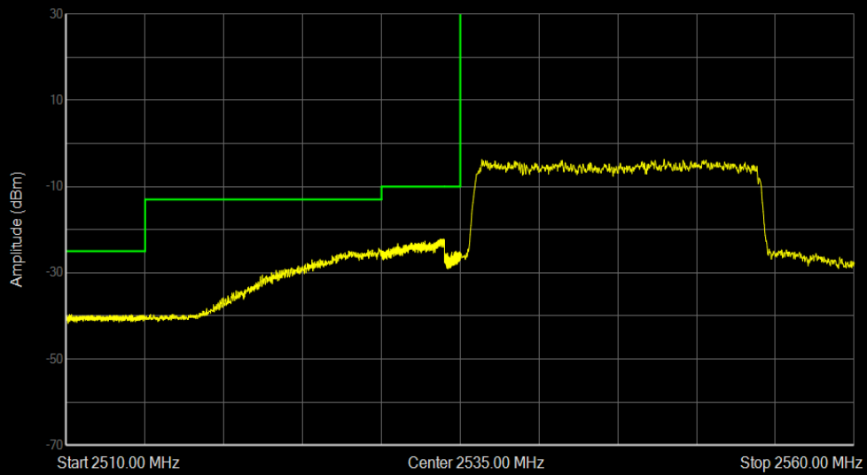
Band41 QPSK BW=20MHz Channel=40140 RB Size=100 Position=#0
