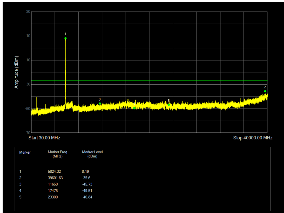
Tx. Spurious NVNT 802.11a 5825MHz Ant1 Emission
