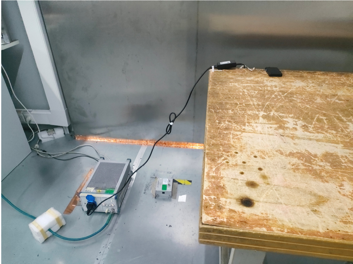
Conducted Emissions - Front View
