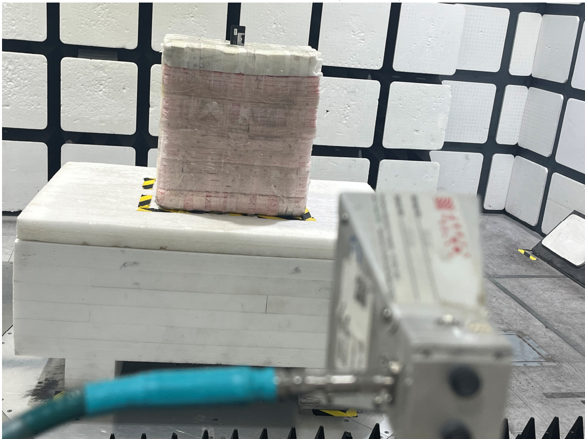
Radiated Emissions View (18-40GHz)
