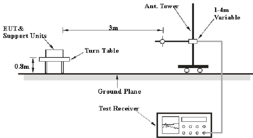
The radiated emission tests were performed in the 3meters test site, using the setup accordance with the ANSI C63.10-2020. The specification used was the FCC 15.205, FCC 15.209, FCC 15.247 limits.
