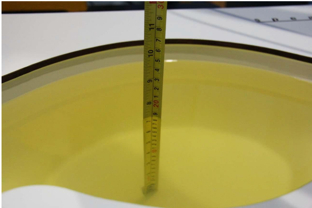
Picture 7-1: Liquid depth in the Flat Phantom(2450MHz)
